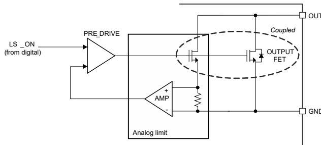
**Figure 6-9. Analog Current Limit and Sensing Diagram**
