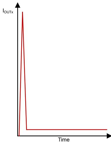
**Figure 6-6. High Startup Current Without Current Limiting Protection**
