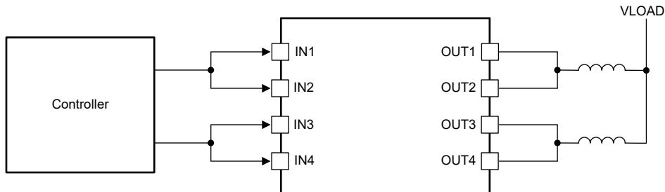
**Figure 6-14. Drive Two Solenoids with Higher Current**
