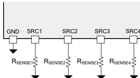
**Figure 6-1. Sense Resistors on Each SRC Pin**
