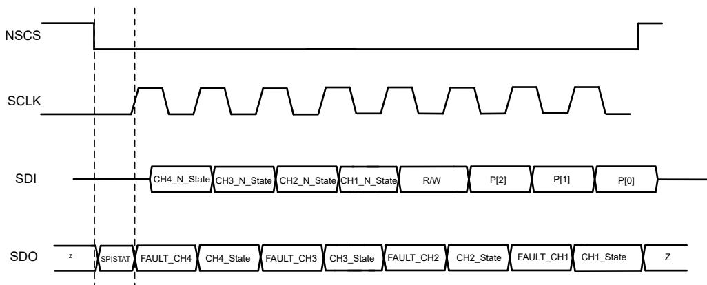
**Figure 6-15. SPI Data - Standard 8-Bit Frame With SPISTAT**
