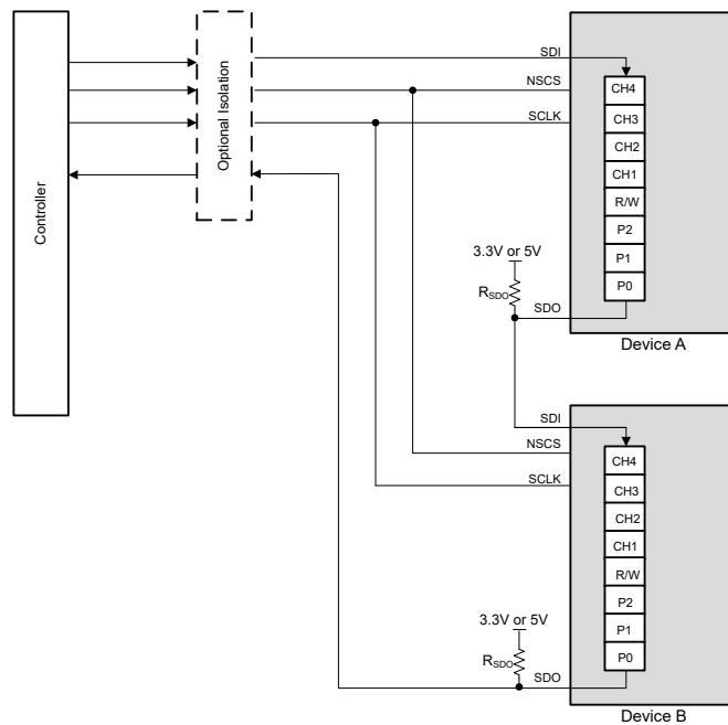
**Figure 6-16. Two DRV81646 Devices Connected in Daisy Chain**
