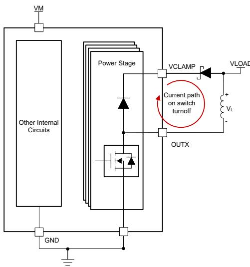
Figure 6-4. Fastest Decay (TVS/Zener VCLAMP to VLOAD)
