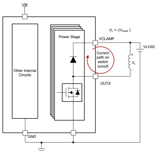
Figure 6-3. Slow Decay (VCLAMP Tied to VLOAD)
