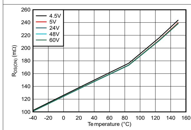
**Figure 5-4.  $R_{DS(on)}$  Over Temperature**
