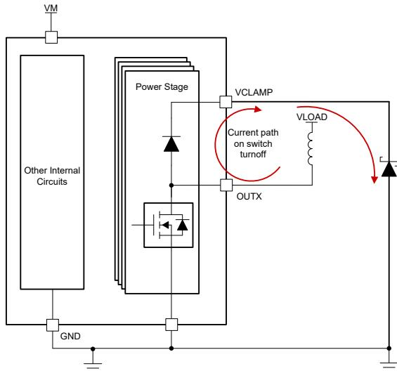
Figure 6-5. Fast Decay (TVS/Zener CLAMP to GND)
