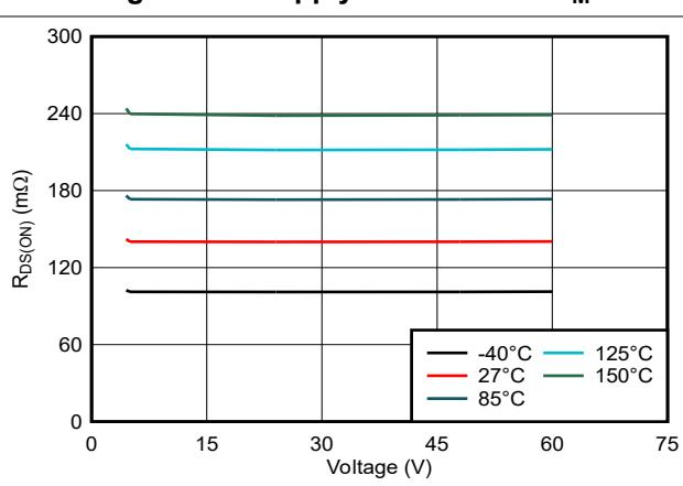
**Figure 5-5.  $R_{DS(on)}$  Over  $V_M$**
