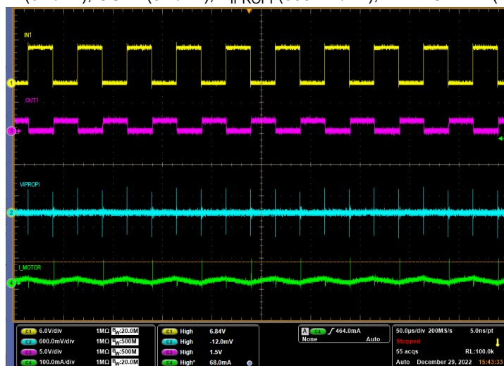
Figure 9-6. PWM Operation at VM = 1.65 V
