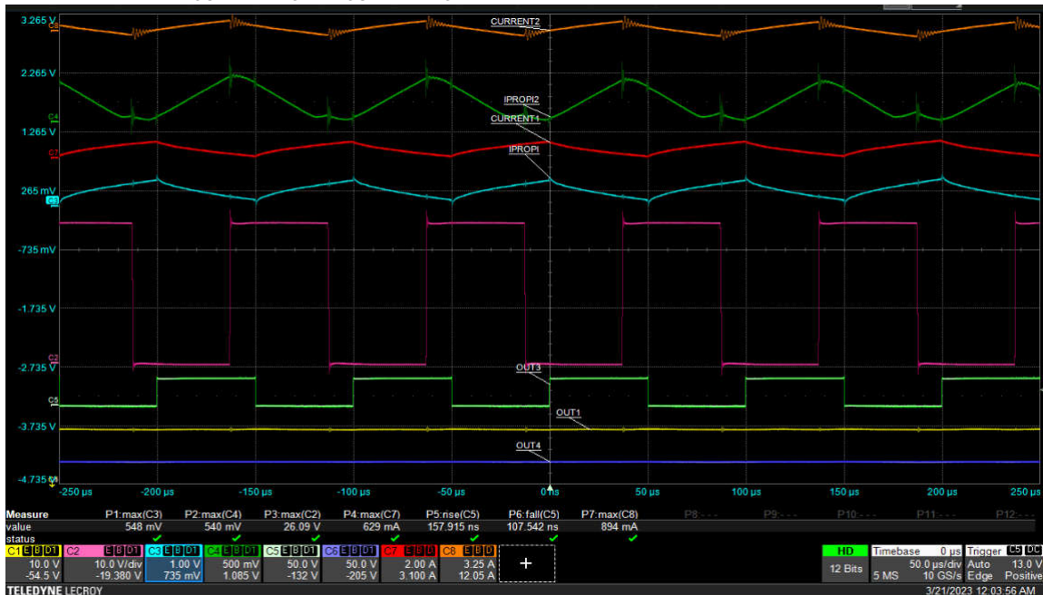
Figure 8-4. Dual H-bridge Operation, V_M = 24 V
