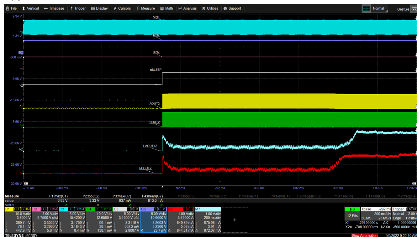
Figure 10-9. No Current Regulation
