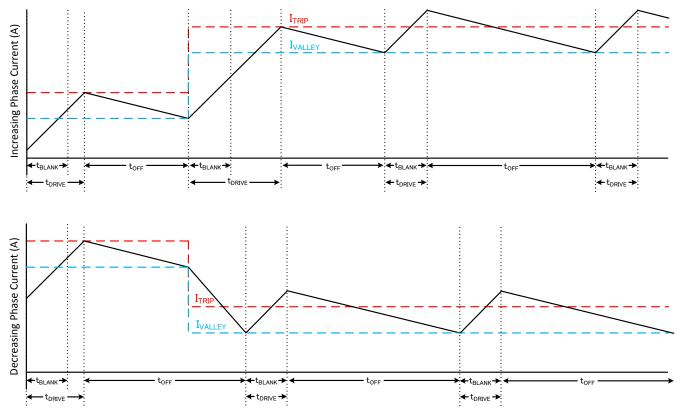
Figure 7-9. Smart tune Ripple Control Decay Mode
