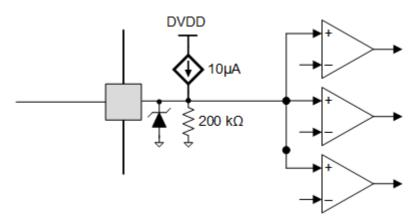
Figure 7-13. Quad-Level Input Pin Diagram
