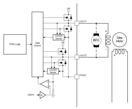
Figure 7-4. PWM Motor Driver Block Diagram
