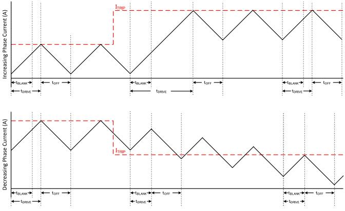
Figure 7-7. Fast/Fast Decay Mode
