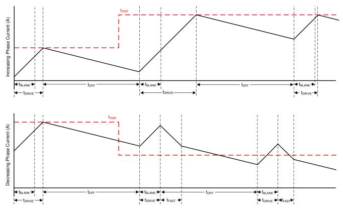
Figure 7-8. Smart tune Dynamic Decay Mode
