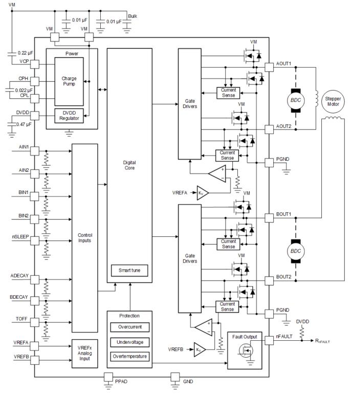
Figure 7-2. DRV8426P Block Diagram
