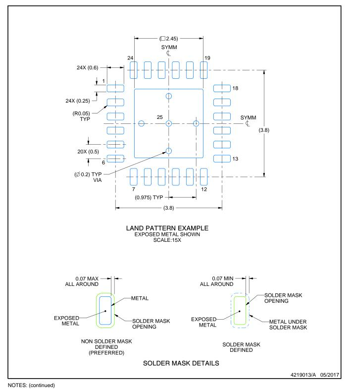
This package is designed to be soldered to a thermal pad on the board. For more information, see Texas Instruments literature number SLUA271 (www.ti.com/lit/slua271).
