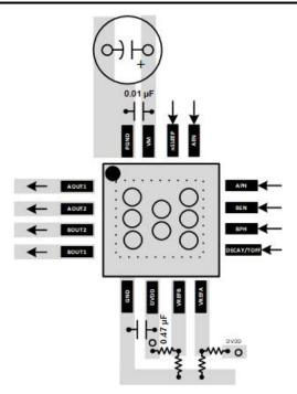
Figure 10-2. QFN Layout Example
