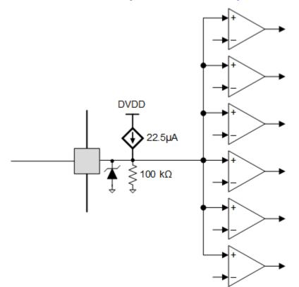
Figure 7-11. Seven-Level Input Pin Diagram
