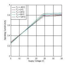
Figure 6-3. Operating Current over Supply Voltage
