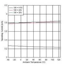
Figure 6-4. Operating Current over Temperature
