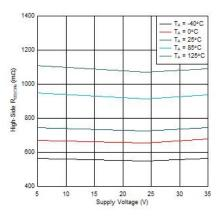
Figure 6-7. High-Side R<sub>DS(ON)</sub> over Supply Voltage
