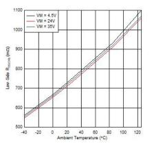
Figure 6-6. Low-Side R<sub>DS(ON)</sub> over Temperature
