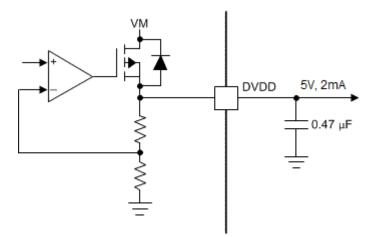
Figure 7-9. Linear Voltage Regulator Block Diagram
