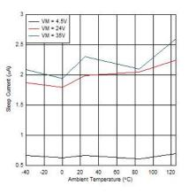
Figure 6-2. Sleep Current over Temperature
