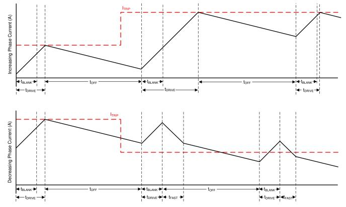
Figure 7-7. Smart tune Dynamic Decay Mode
