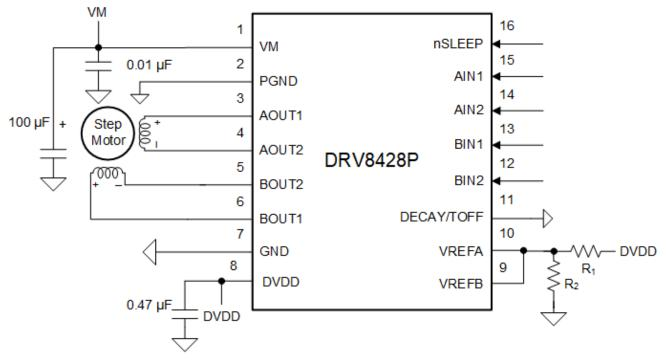
Figure 8-3. Typical Application Schematic
