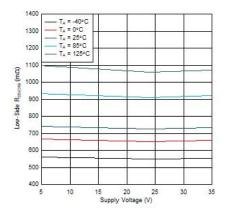
Figure 6-5. Low-Side R<sub>DS(ON)</sub> over Supply Voltage
