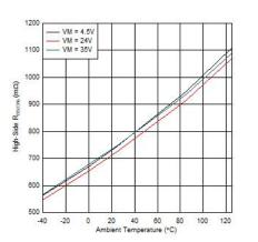
Figure 6-8. High-Side R<sub>DS(ON)</sub> over Temperature
