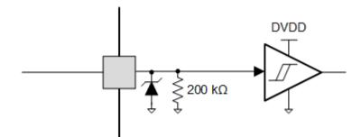
Figure 7-10. Logic-level Input Pin Diagram
