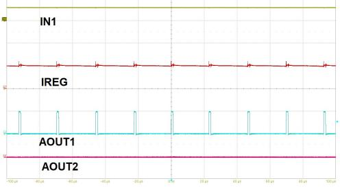
Figure 8-2. Driver Full On Operation with Current Regulation
