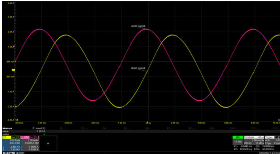
Figure 7-21. Coil Current Waveform with Silent Step Decay
