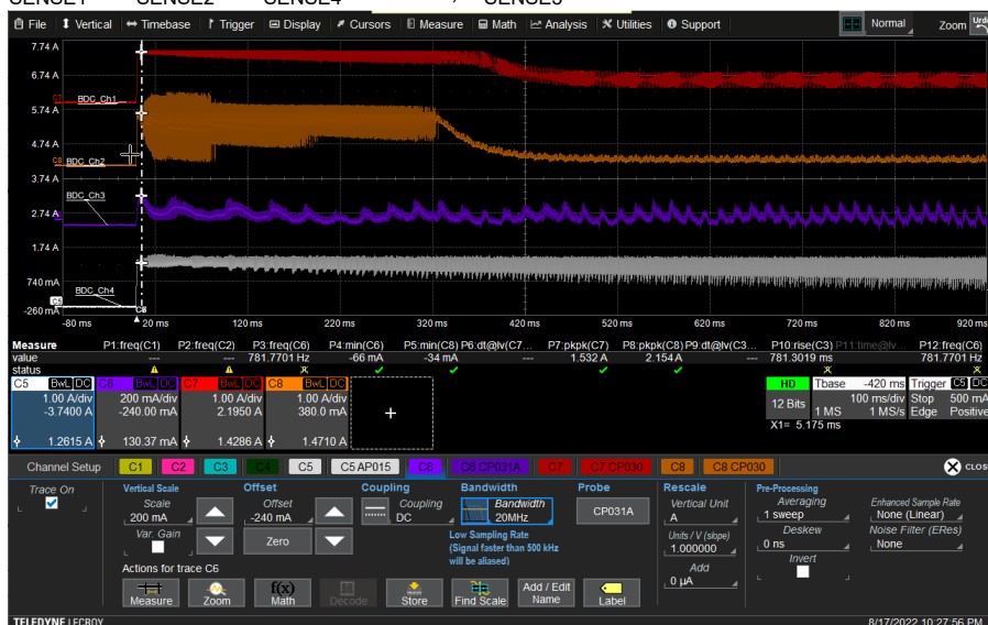
Figure 8-3. Driving four brushed-DC motors
