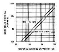
Figure 6. Noise Pulse Width vs Response Control Capacitor
