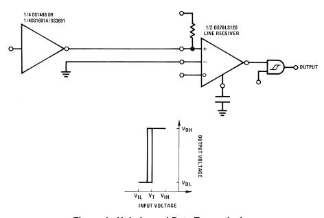
Figure 4. Unbalanced Data Transmission
