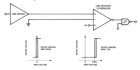
Figure 9. Balanced RS-422 Fail-Safe
