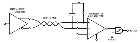
Figure 3. Balanced Data Transmission
