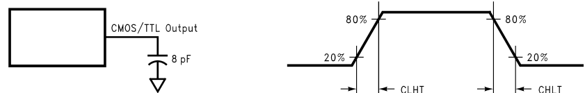
Figure 4. Receiver CMOS/TTL Output Load and Transition Times
