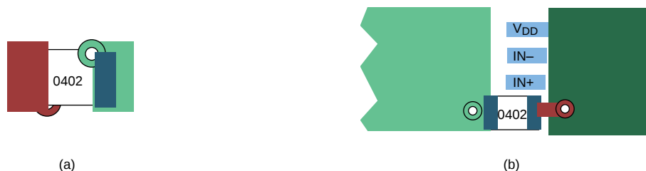
Figure 27. Typical Decoupling Capacitor Layouts
