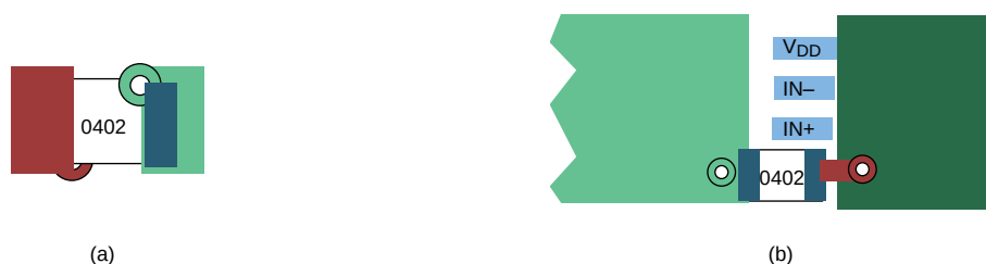
Figure 21. Typical Decoupling Capacitor Layouts
