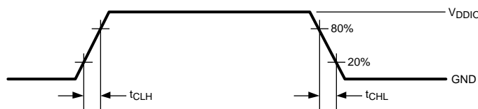
Figure 3. LVC MOS Transition Times
