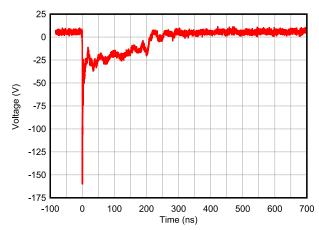
Figure 8-2. +8-kV Clamped IEC Waveform
