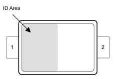
Figure 5-2. DYA Package, 2-Pin SOD523 (Top View)
