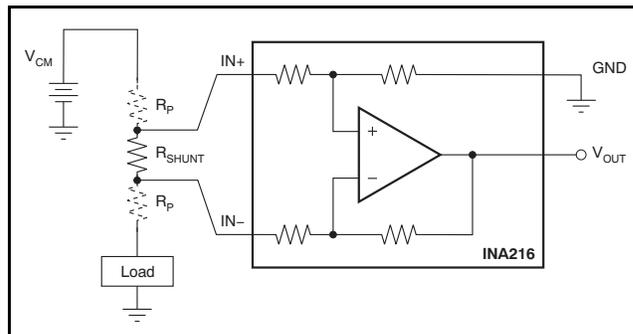
Figure 20. Shunt Resistance Measurement Using a Kelvin Connection
