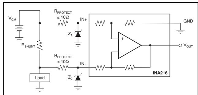
**Figure 22. Transient Protection Using Dual Zener Diodes**
