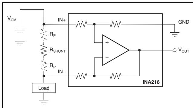
Figure 19. Shunt Resistance Measurement Including Trace Resistance,  $R_P$
