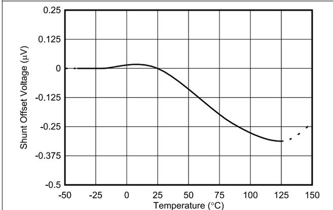
Figure 6-4. Shunt Input Offset Voltage vs. Temperature
