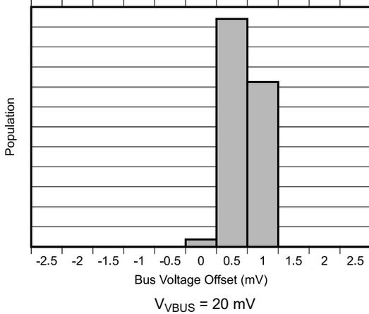
**Figure 6-10. Bus Input Offset Voltage Production Distribution**
