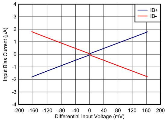
Figure 6-14. Input Bias Current vs. Differential Input Voltage
