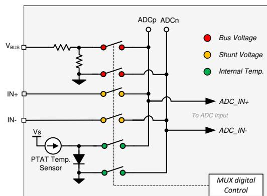
Figure 7-1. High-Voltage Input Multiplexer
