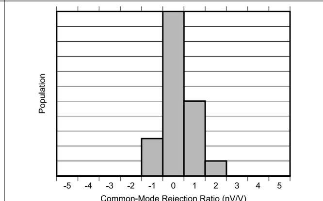
Figure 6-5. Common-Mode Rejection Ratio Production Distribution
