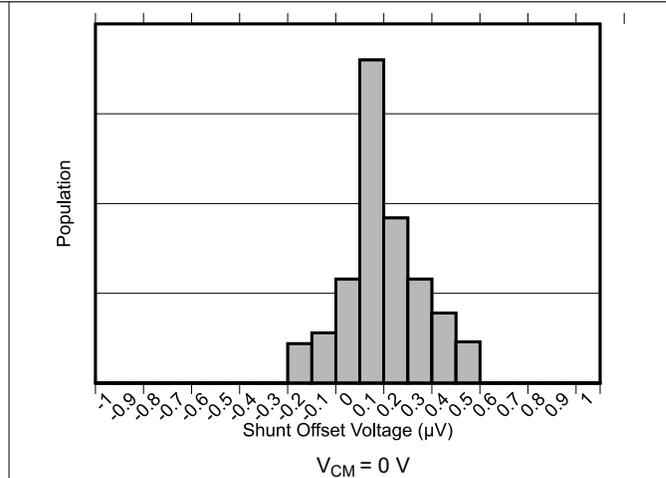
Figure 6-3. Shunt Input Offset Voltage Production Distribution
