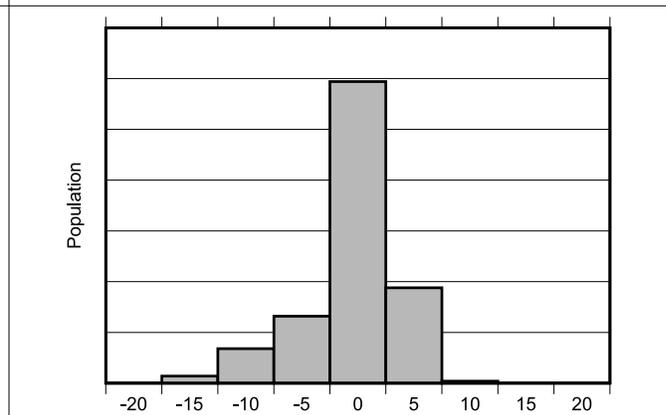
Figure 6-7. Shunt Input Gain Error Production Distribution
