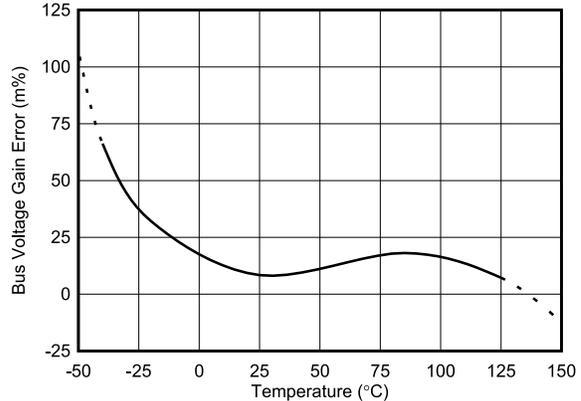
**Figure 6-13. Bus Input Gain Error vs. Temperature**
