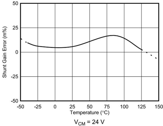
**Figure 6-8. Shunt Input Gain Error vs. Temperature**
