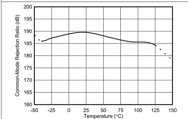
Figure 6-6. Shunt Input Common-Mode Rejection Ratio vs. Temperature
