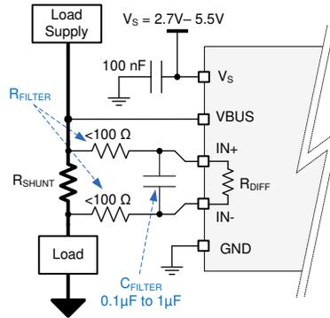
Figure 8-1. Input Filtering
