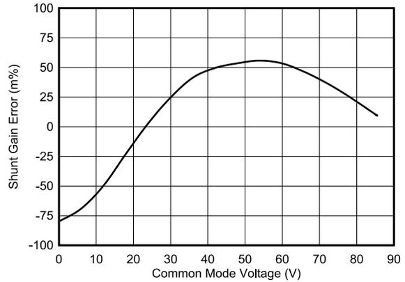
**Figure 6-9. Shunt Input Gain Error vs. Common-Mode Voltage**
