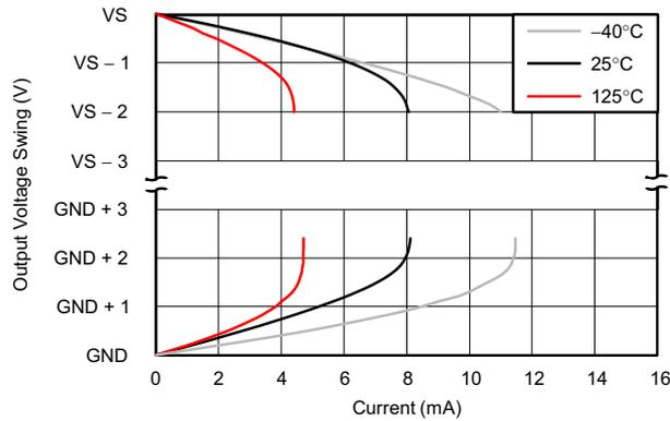
**Figure 6-19. Output Voltage Swing vs Output Current**
