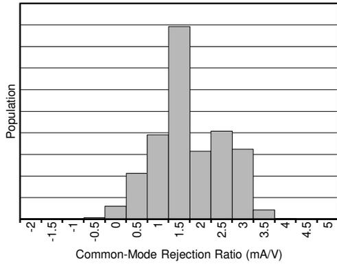
**Figure 6-7. INA250A2 Common-Mode Rejection Ratio Distribution**
