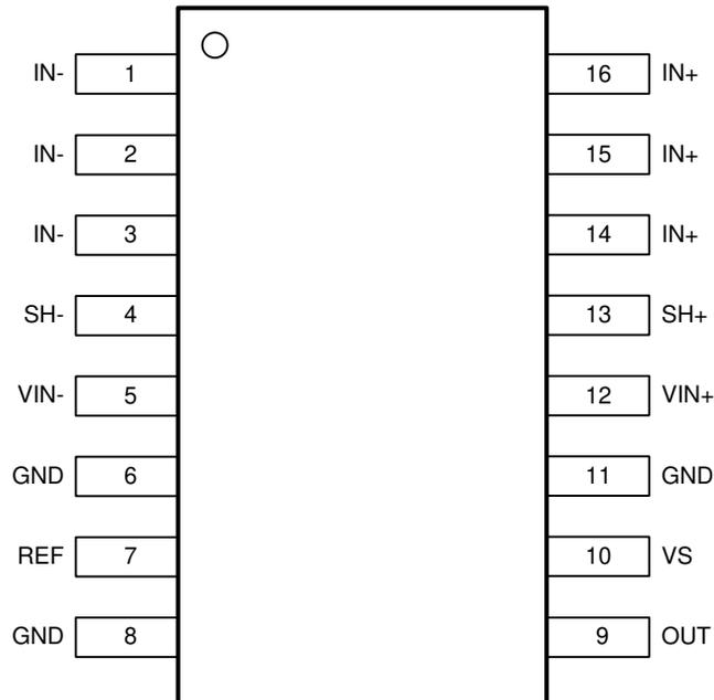
**Figure 5-1. PW Package 16-Pin TSSOP Top View**
