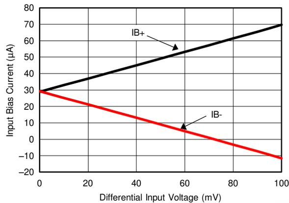
Figure 7-5. Input Bias Current vs Differential Input Voltage
