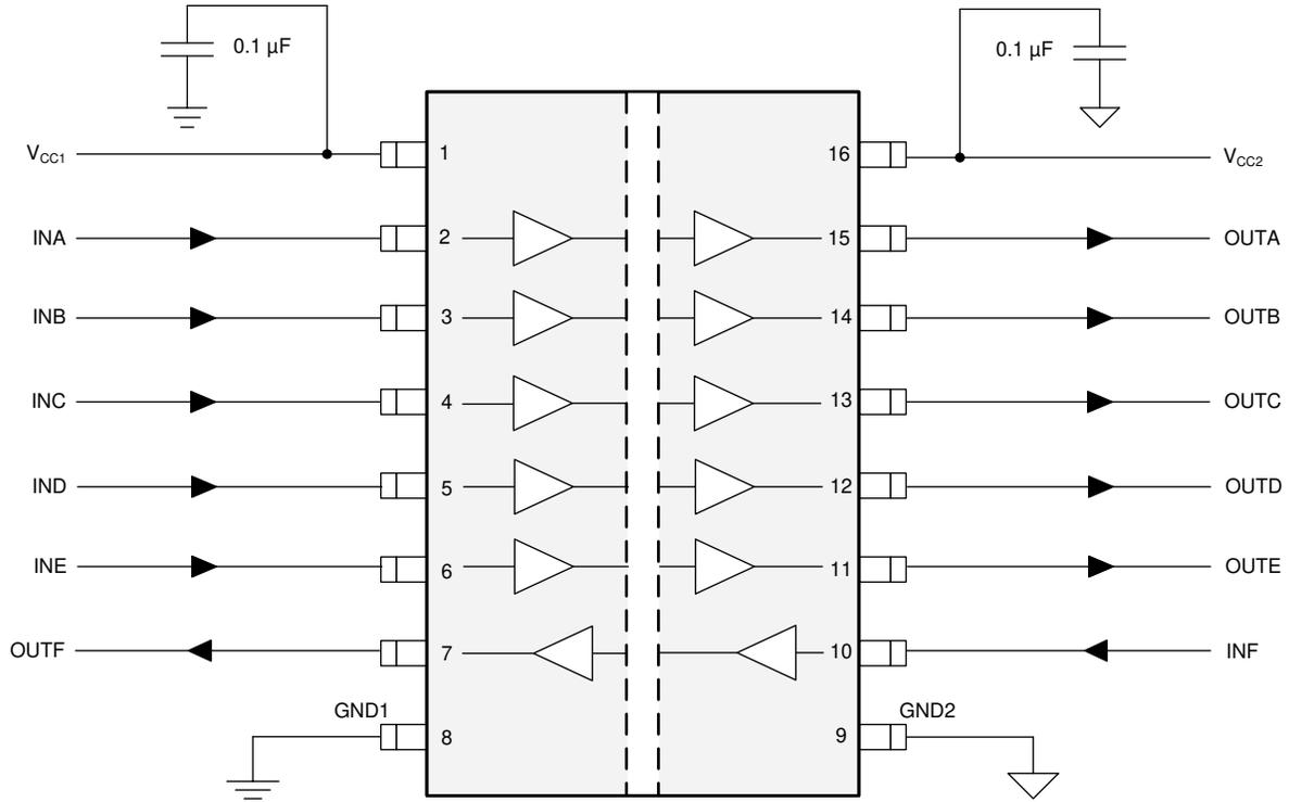
Figure 8-2. Typical ISO7761 Circuit Hook-up
