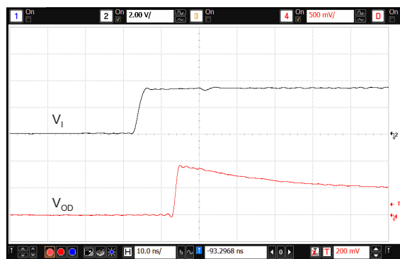
Figure 15. Distortion Correction Scheme Calibration Time ( t_{CALIB} )
