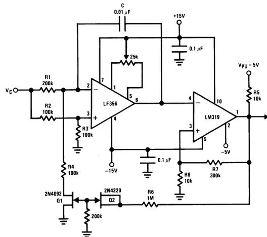
$$f = \frac{V_C (R_8 + R_7)}{(8 V_{PU} R_8 R_1) C'} \quad 0 \leq V_C \leq 30\text{V}, \quad 10 \text{ Hz} \leq f \leq 10 \text{ kHz}$$
