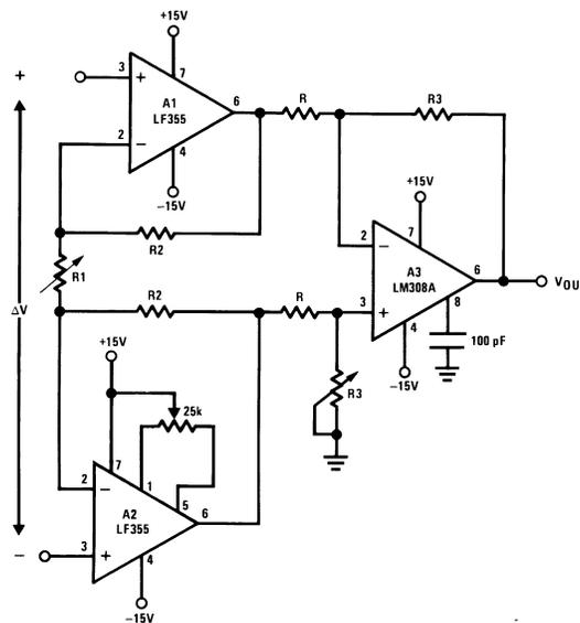
$$V_{OUT} = \frac{R3}{R} \left[ \frac{2R2}{R1} + 1 \right] \Delta V, \quad V^- + 2V \leq V_{IN \text{ common-mode}} \leq V^+$$
