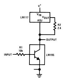
Figure 28. High Gain Amplifier
