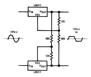
Figure 35. AC Voltage Regulator
