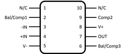
Pin connections shown on schematic diagram and typical applications are for TO package.
