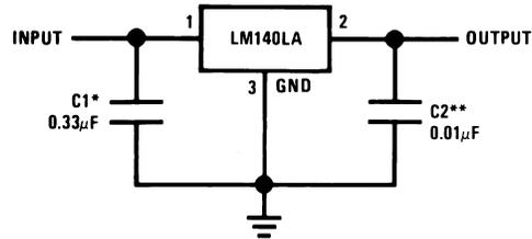
\*Required if the regulator is located far from the power supply filter.
