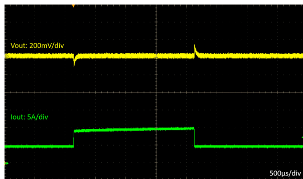
Figure 7-12. Load Transient, 5A to 10A
