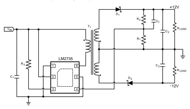
Figure 34. LM2735Y-Q1 (520 kHz):  $V_{IN}$  = 5 V,  $V_{OUT}$  = ±12 V 150 mA
