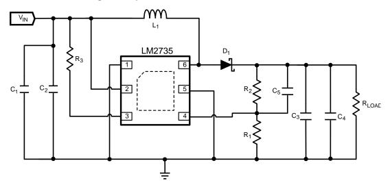
Figure 24. LM2735X-Q1 (1.6 MHz):  $V_{IN}$  = 3.3 V,  $V_{OUT}$  = 12 V at 350 mA
