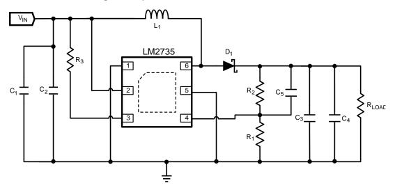
Figure 31. LM2735Y-Q1 (520 kHz):  $V_{IN}$  = 3.3 V,  $V_{OUT}$  = 20 V at 150 mA
