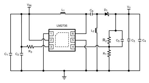
Figure 37. SEPIC Converter Schematic
