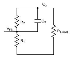
Figure 17. Setting External Pole-Zero
