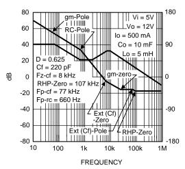
Figure 16. LM2735-Q1 With External Compensation
