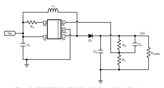
Figure 18. LM2735X-Q1 (1.6 MHz):  $V_{IN} = 5 \text{ V}$ ,  $V_{OUT} = 12 \text{ V}$  at 350 mA
