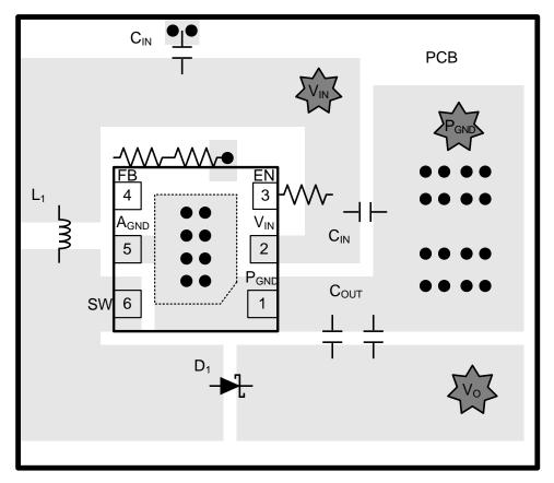
Figure 42. Example of Proper PCB Layout
