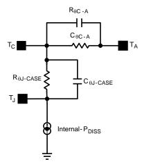
Figure 44. Simplified Thermal Impedance Model
