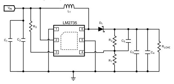
Figure 25. LM2735Y-Q1 (520 kHz):  $V_{IN}$  = 3.3 V,  $V_{OUT}$  = 12 V at 350 mA
