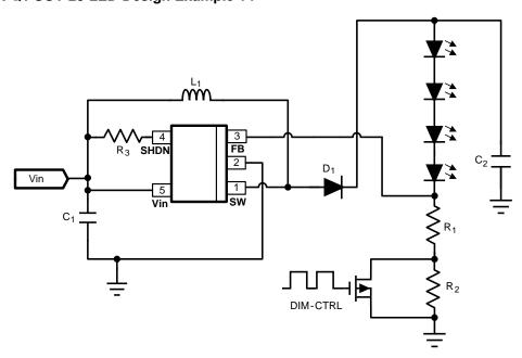
Figure 33. LM2735X-Q1 (1.6 MHz):  $V_{IN}$  = 2.7 V - 5 V,  $V_{OUT}$  = 20 V at 50 mA
