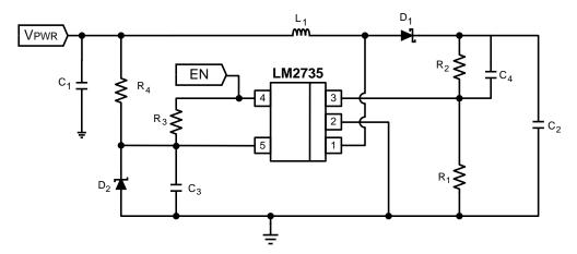
Figure 35. LM2735X-Q1 (1.6 MHz):  $V_{PWR} = 9 \text{ V}$ ,  $V_{OUT} = 12 \text{ V}$  at 500 mA
