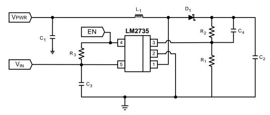
Figure 36. LM2735X-Q1 (1.6 MHz):  $V_{PWR} = 9 \ V_{IN} = 2.7 \ V - 5.5 \ V$ ,  $V_{OUT} = 12 \ V$  at 500 mA
