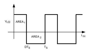
Figure 38. Inductor Volt-Sec Balance Waveform
