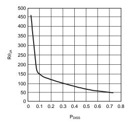
Figure 48. R<sub>θJA</sub> vs Internal Dissipation for the WSON
