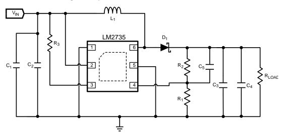
Figure 30. LM2735X-Q1 (1.6 MHz):  $V_{IN} = 3.3 \text{ V}$ ,  $V_{OUT} = 20 \text{ V}$  at 150 mA
