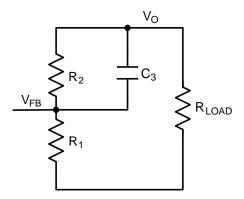
Figure 20. Setting V<sub>OUT</sub>
