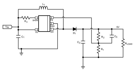
Figure 26. LM2735-Q1X (1.6 MHz):  $V_{IN} = 3 \text{ V}$ ,  $V_{OUT} = 5 \text{ V}$  at 500 mA
