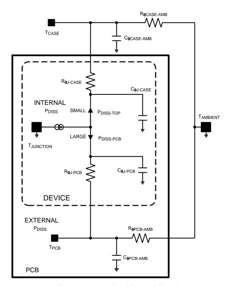
Figure 46. Associated Thermal Model
