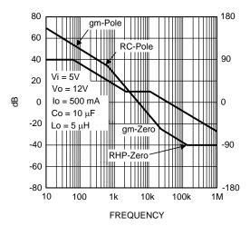
Figure 15. LM2735-Q1 Without External Compensation
