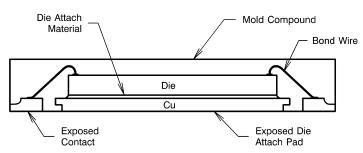
Figure 40. Internal WSON Connection
