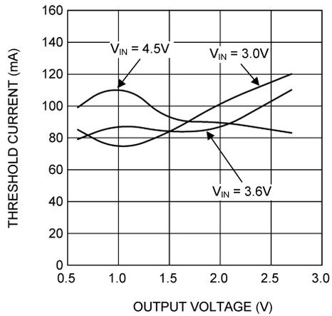
Figure 9. ECO-PWM Mode Threshold Current vs Output voltage
