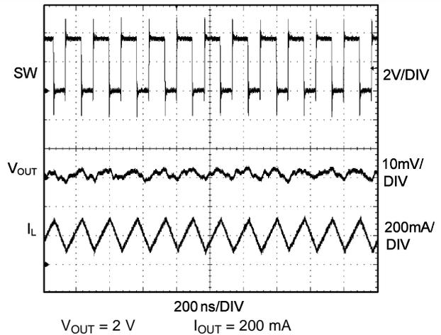
Figure 20. Output Voltage Ripple in PWM Mode
