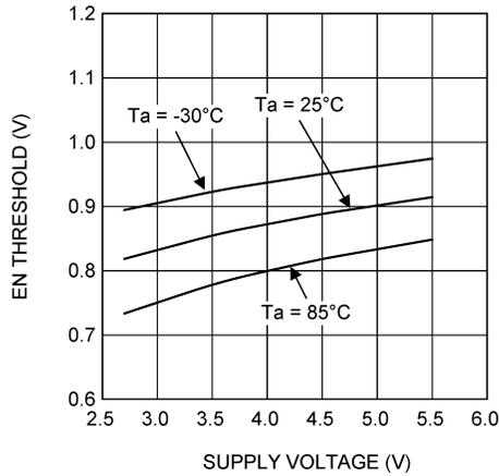
Figure 19. EN High Threshold vs Supply Voltage
