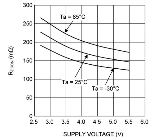
Figure 15. PFET  $R_{DS(on)}$  vs Supply Voltage
