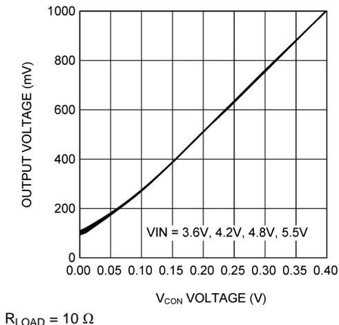
Figure 17. Low  $V_{CON}$  Voltage vs Output Voltage
