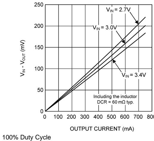
Figure 18.  $V_{IN} - V_{OUT}$  vs Output Current
