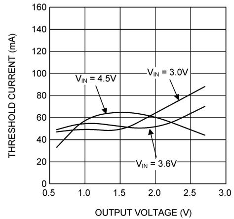
Figure 10. PWM-Eco-Mode Threshold Current vs Output voltage
