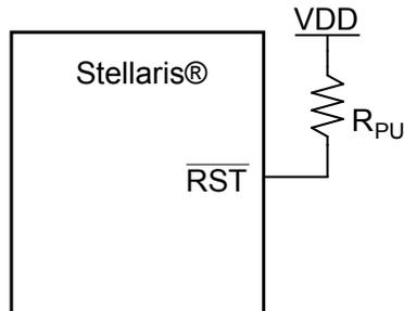
$R_{\text{PU}} = 0$  to 100 k $\Omega$
