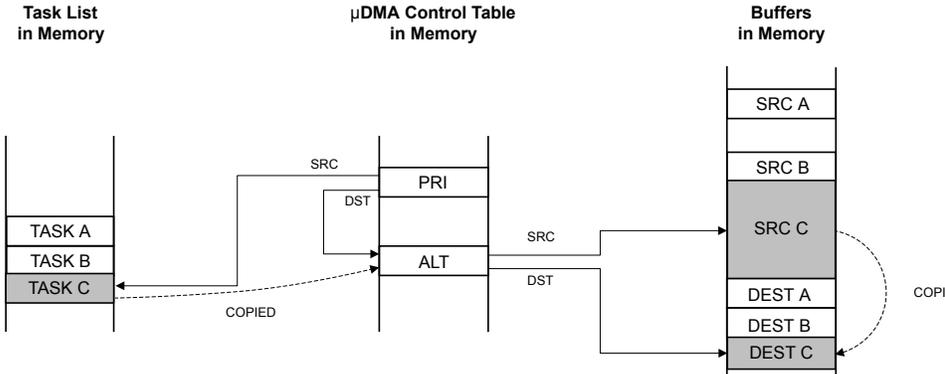
Using the channel's primary control structure, the  $\mu$ DMA controller copies task C configuration to the channel's alternate control structure.
