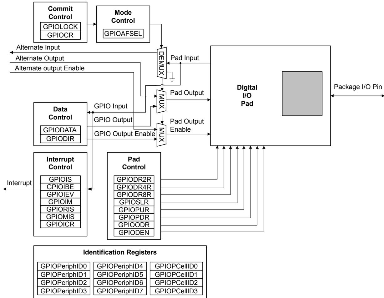
Figure 8-2. Analog/Digital I/O Pads
