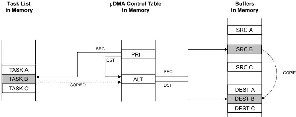
Using the channel's primary control structure, the  $\mu$ DMA controller copies task B configuration to the channel's alternate control structure.
