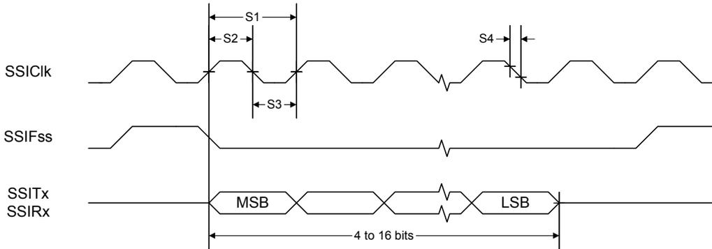
**Figure 20-11. SSI Timing for MICROWIRE Frame Format (FRF=10), Single Transfer**
