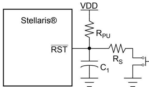
Typical  $R_{PU} = 10 \text{ k}\Omega$
