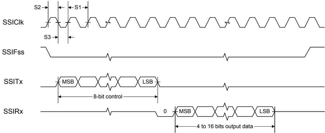
Figure 20-12. SSI Timing for SPI Frame Format (FRF=00), with SPH=1
