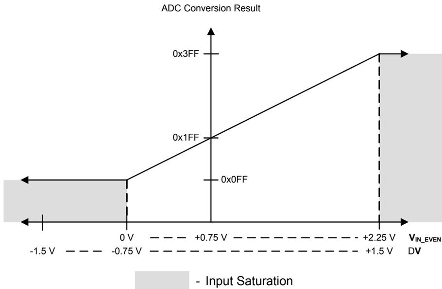
Figure 11-4. Differential Sampling Range,  $V_{IN\_ODD} = 2.25\text{ V}$
