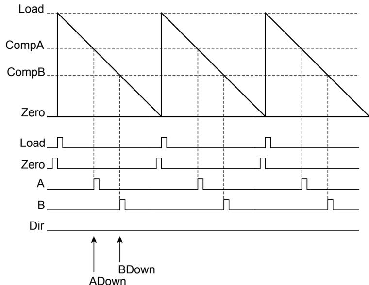
**Figure 19-4. PWM Count-Up/Down Mode**
