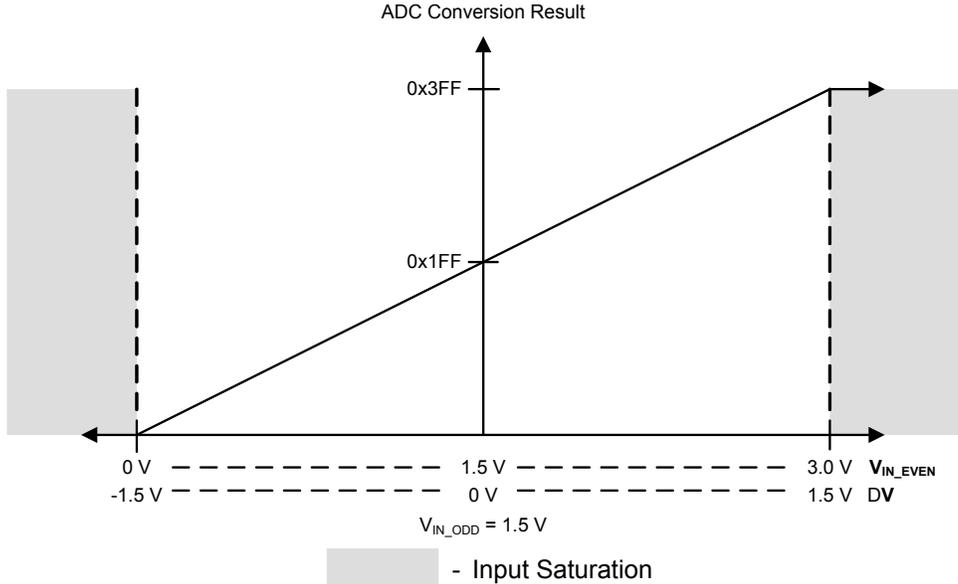
Figure 12-3. Differential Sampling Range,  $V_{IN\_ODD} = 0.75\text{ V}$
