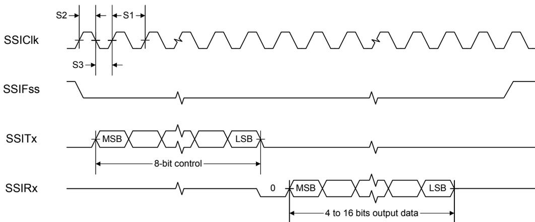
Figure 24-13. SSI Timing for SPI Frame Format (FRF=00), with SPH=1
