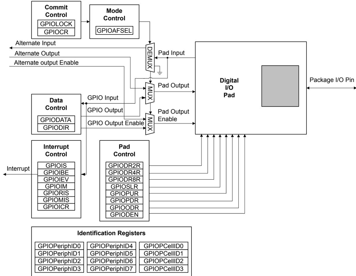
Figure 9-2. Analog/Digital I/O Pads
