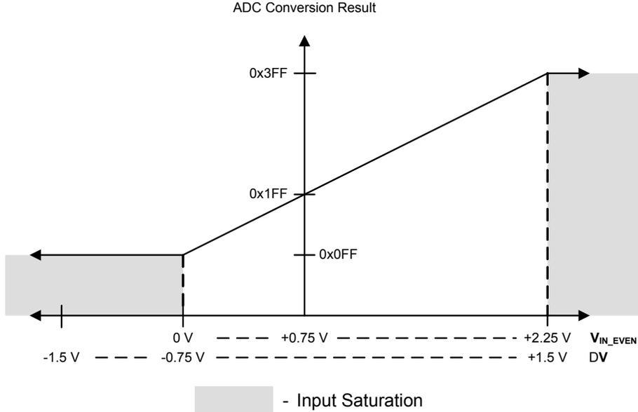
Figure 12-4. Differential Sampling Range,  $V_{IN\_ODD} = 2.25\text{ V}$
