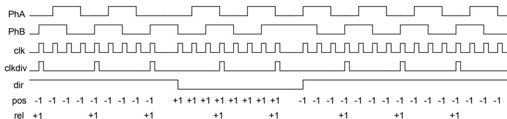
The period of the timer is configurable by specifying the load value for the timer in the **QEILOAD** register. When the timer reaches zero, an interrupt can be triggered, and the hardware reloads the
