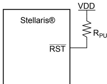
$R_{\text{PU}} = 0$  to 100 k $\Omega$
