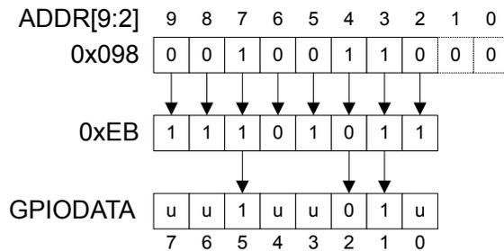
During a read, if the address bit associated with the data bit is set to 1, the value is read. If the address bit associated with the data bit is set to 0, it is read as a zero, regardless of its actual value. For example, reading address **GPIO DATA** + 0x0C4 yields as shown in Figure 9-4 on page 373.
