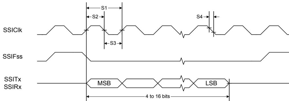
Figure 20-12. SSI Timing for MICROWIRE Frame Format (FRF=10), Single Transfer
