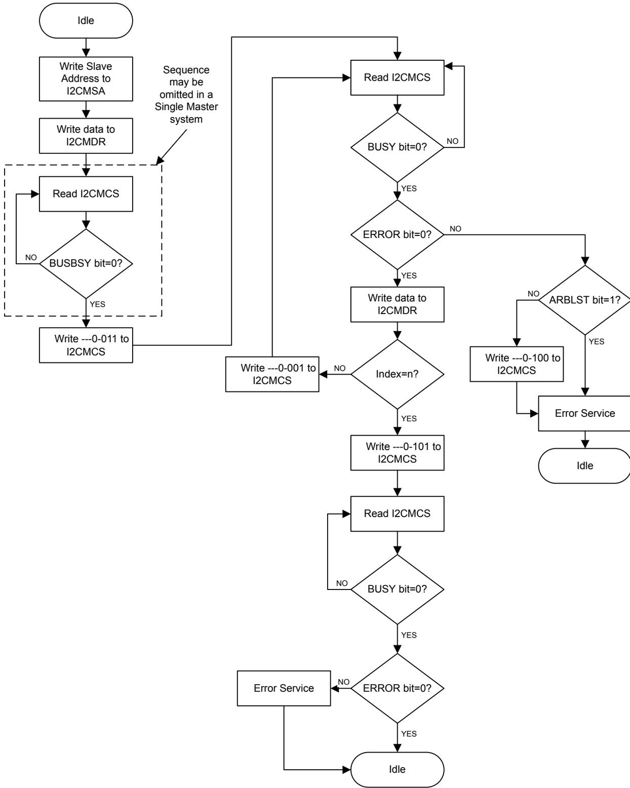
Figure 13-10. Master Burst RECEIVE
