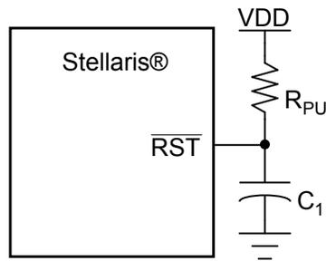
$$R_{PU} = 1 \text{ k}\Omega \text{ to } 100 \text{ k}\Omega$$
