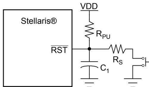
$$\text{Typical } R_{PU} = 10 \text{ k}\Omega$$
