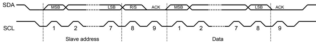
The first seven bits of the first byte make up the slave address (see Figure 13-5 on page 484). The eighth bit determines the direction of the message. A zero in the R/S position of the first byte means that the master will write (send) data to the selected slave, and a one in this position means that the master will receive data from the slave.
