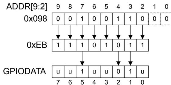
During a read, if the address bit associated with the data bit is set to 1, the value is read. If the address bit associated with the data bit is set to 0, it is read as a zero, regardless of its actual value. For example, reading address GPIODATA + 0x0C4 yields as shown in Figure 7-3 on page 252.
