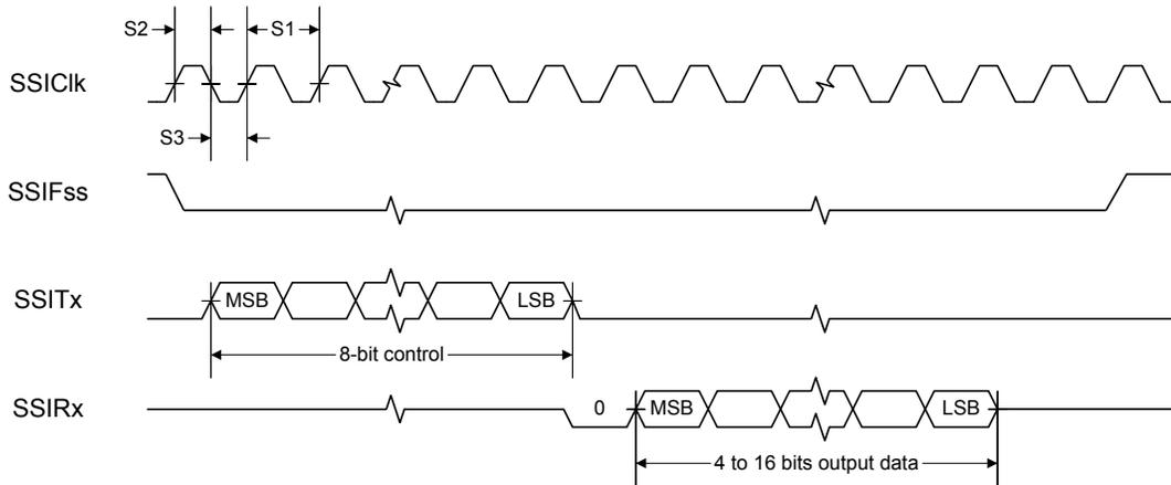
Figure 17-12. SSI Timing for SPI Frame Format (FRF=00), with SPH=1
