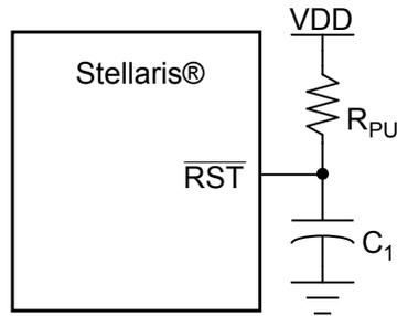
$R_{PU} = 1 \text{ k}\Omega \text{ to } 100 \text{ k}\Omega$
