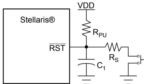
Typical  $R_{PU} = 10 \text{ k}\Omega$
