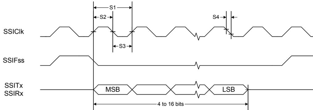
**Figure 17-11. SSI Timing for MICROWIRE Frame Format (FRF=10), Single Transfer**
