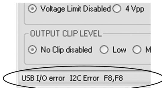
Figure 62. Error Message displayed on GUI if device is NOT acknowledged (I<sup>2</sup>C Error) or if there is an USB error (USB I/O error)
