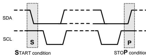
Figure 49. I<sup>2</sup>C Start and Stop Conditions
