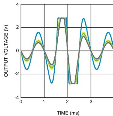
Figure 57. Clip Control Levels
