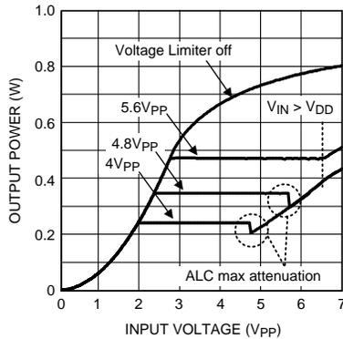
**Figure 58. Voltage Limiter Function**
