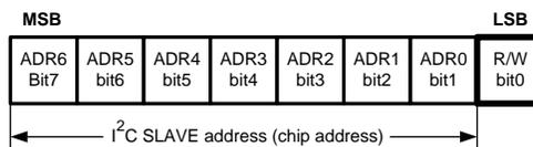
Figure 50. I<sup>2</sup>C Chip Address
