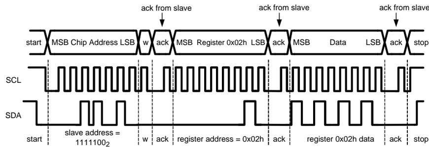
Figure 51. Example I<sup>2</sup>C Write Cycle
