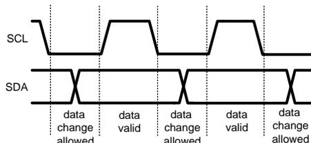
Figure 48. I<sup>2</sup>C Signals: Data Validity
