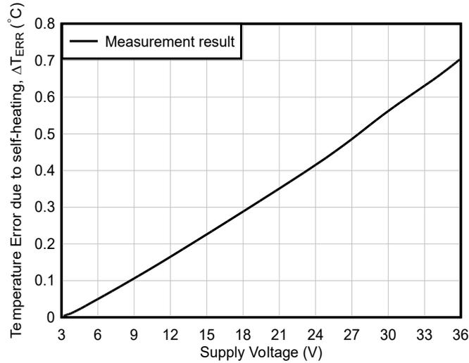
The device soldered to 30 gauge wire. The accuracy is read after consistently 10min working of the device at 25°C.
