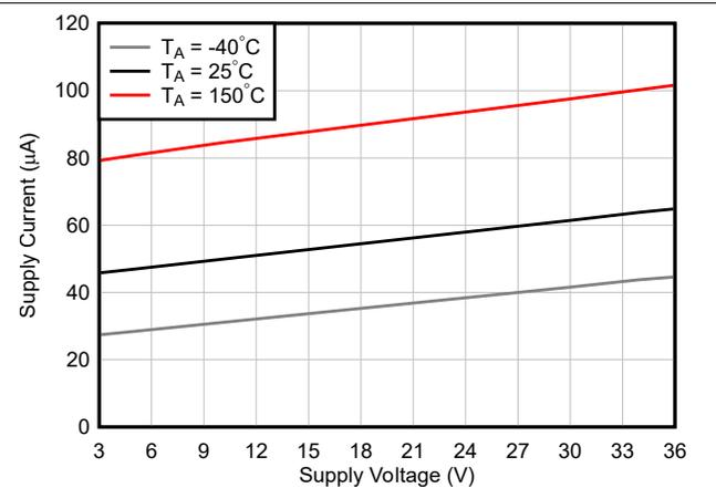
**Figure 6-26. Supply Current vs Supply Voltage**
