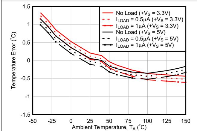
**Figure 6-23. Accuracy vs Ambient Temperature with different loads**
