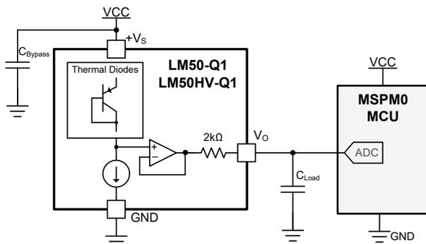
Figure 3-1. Simplified Schematic
