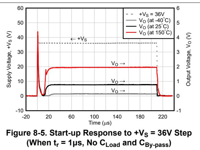
Figure 8-5. Start-up Response to +V<sub>S</sub> = 36V Step (When t<sub>r</sub> = 1μs, No C<sub>Load</sub> and C<sub>By-pass</sub>)
