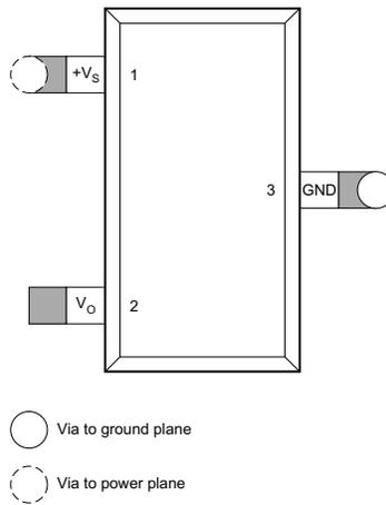
**Figure 8-13. PCB Layout**
