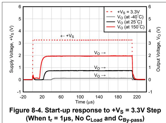
Figure 8-4. Start-up response to +V<sub>S</sub> = 3.3V Step (When t<sub>r</sub> = 1μs, No C<sub>Load</sub> and C<sub>By-pass</sub>)
