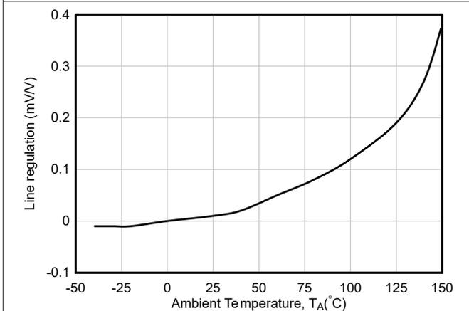
**Figure 6-29. Line Regulation vs Ambient Temperature**
