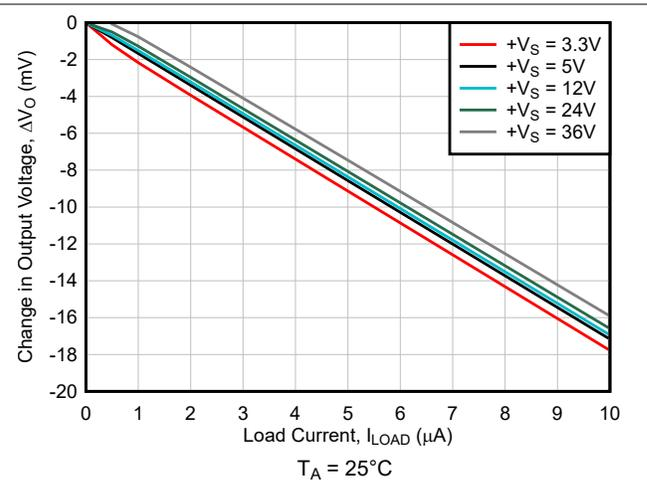
**Figure 6-28. Change in Output Voltage vs Load Current**
