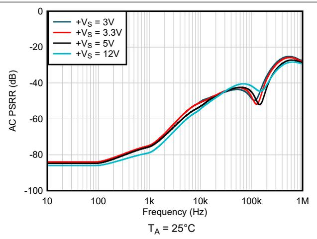
Figure 6-34. Power Supply Rejection Ratio vs Frequency
