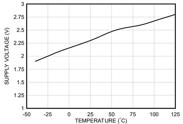
**Figure 6-10. Start-Up Voltage vs Temperature (New chip)**
