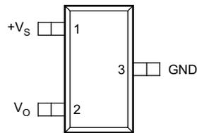
**Figure 5-1. DBZ Package 3-Pin SOT-23 Top View**
