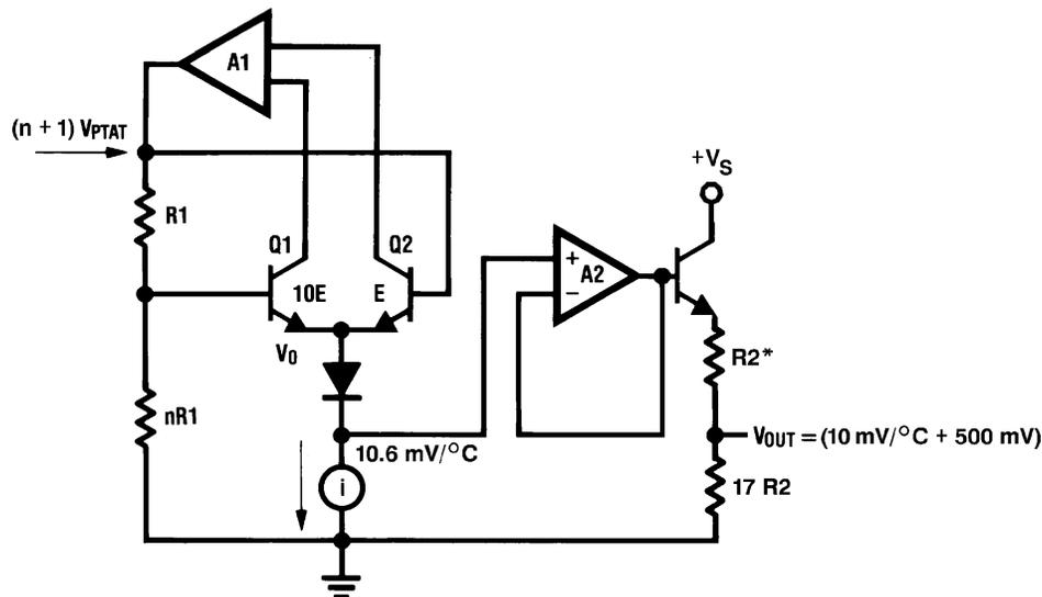
\* $R2 \cong 2\text{k}$  with a typical  $1300\text{ppm}/^{\circ}\text{C}$  drift.
