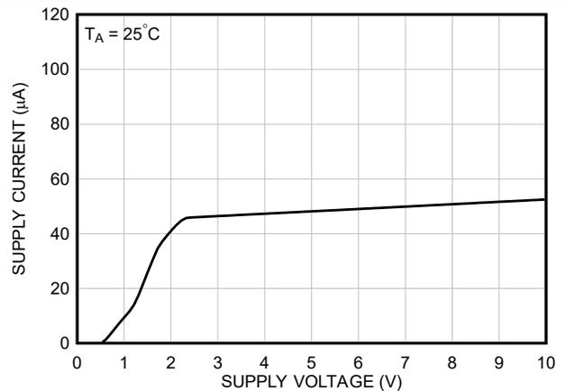
Figure 6-18. Supply Current vs Supply Voltage (New chip)
