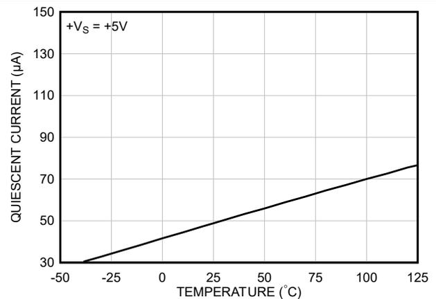
**Figure 6-12. Quiescent Current vs Temperature (New chip)**
