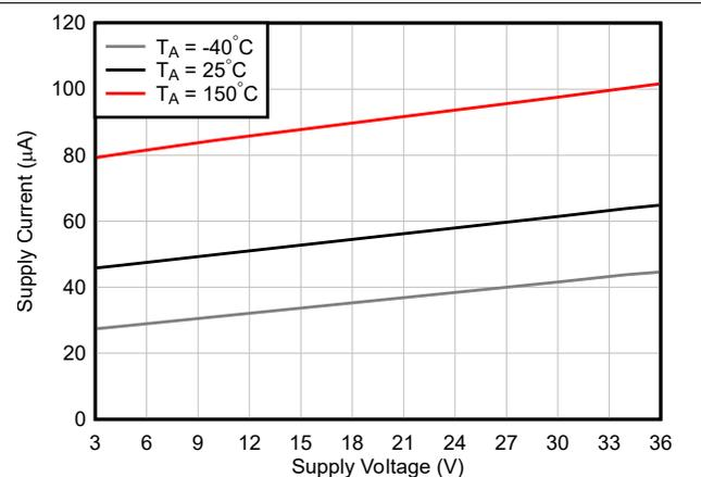
Figure 6-26. Supply Current vs Supply Voltage
