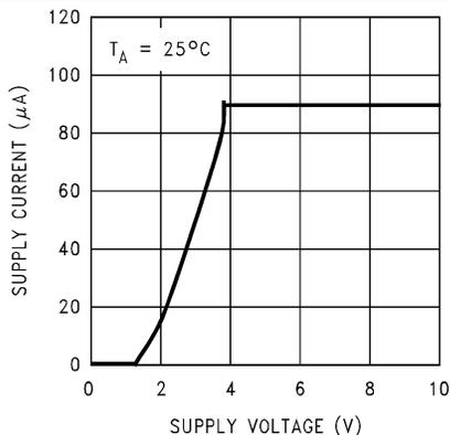
**Figure 6-17. Supply Current vs Supply Voltage (Legacy chip)**
