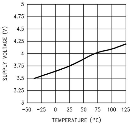
**Figure 6-9. Start-Up Voltage vs Temperature (Legacy chip)**
