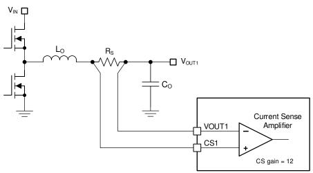
Figure 8-4. Shunt Current Sensing Implementation
