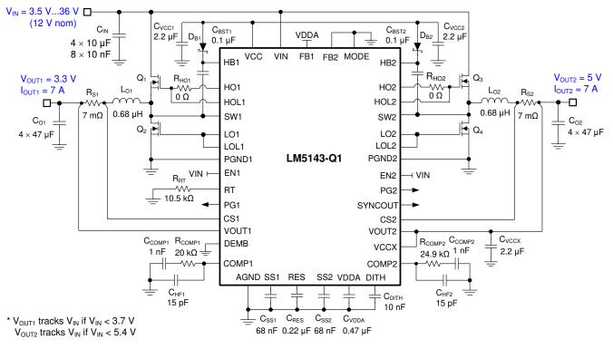
Figure 9-4. Application Circuit 1 With LM5143-Q1 Buck Regulator at 2.1 MHz
