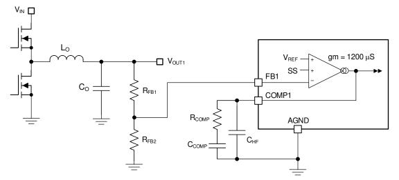
Figure 8-3. Control Loop Error Amplifier
