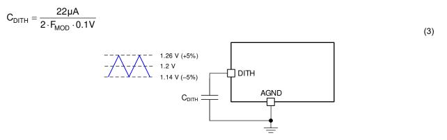
Figure 8-2. Switching Frequency Dithering
