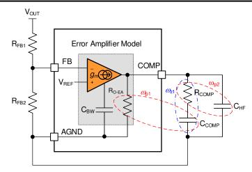
Figure 9-3. Error Amplifier and Compensation Network
