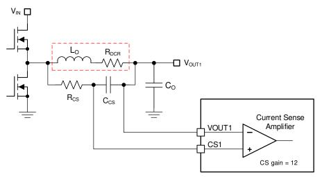
Figure 8-5. Inductor DCR Current Sensing Implementation
