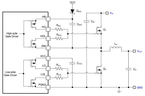
Figure 8-7. Integrated MOSFET Gate Drivers
