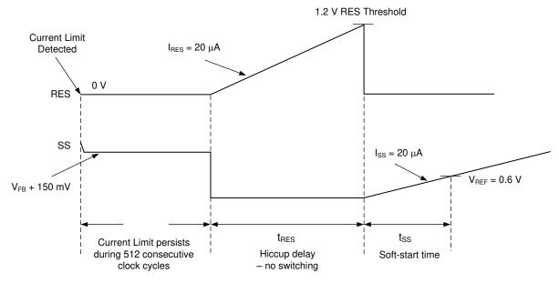
Figure 8-6. Hiccup Mode Timing Diagram
