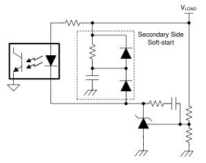
Figure 9-8. Secondary-Side Soft Start in Flyback
