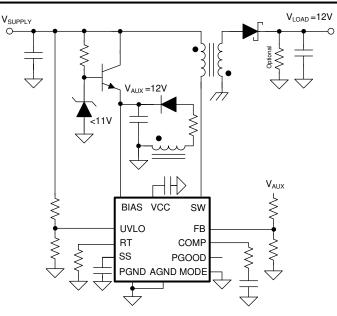
Figure 9-6. External BIAS Supply (PSR Flyback)
