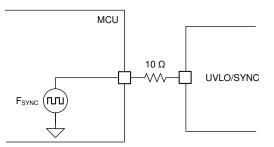
Figure 9-15. Shutdown and Clock Synchronization
