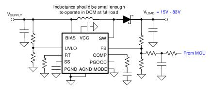
Figure 10-5. LIDAR Bias Supply 1 (DCM Operation)
