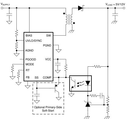
Figure 10-8. Secondary-Side Regulated Isolated Flyback
