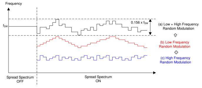
Figure 9-9. Dual Random Spread Spectrum
