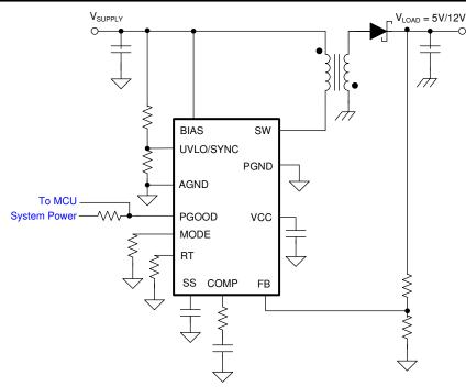
Figure 10-10. Typical Non-Isolated Flyback
