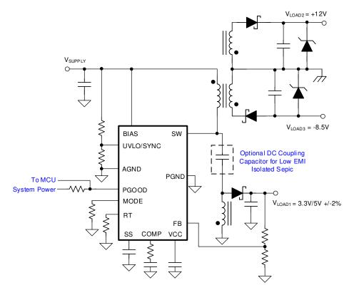
Figure 10-9. Primary-Side Regulated Multiple-Output Isolated Flyback/Isolated SEPIC
