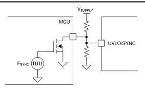
Figure 9-11. UVLO, Shutdown, and Clock Synchronization
