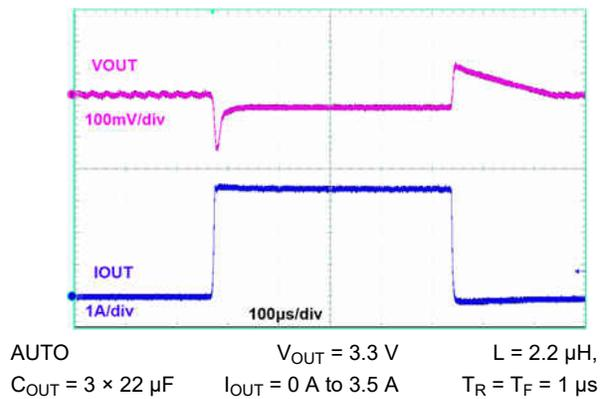
Figure 9-30. Load Transient
