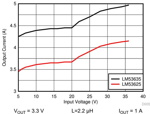
Figure 9-29. Output Current Level for Overcurrent Protection Trip
