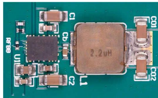
Typical Automotive Layout (22 mm  $\times$  12.5 mm)
