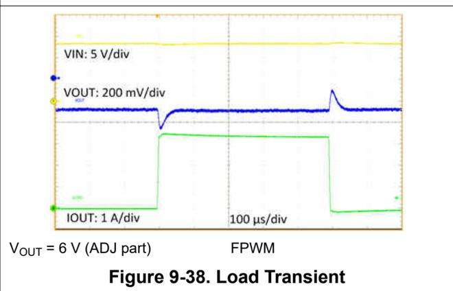
Figure 9-38. Load Transient
