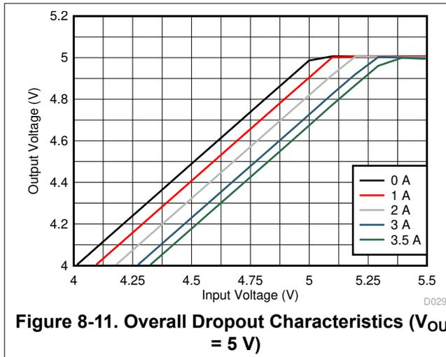
**Figure 8-11. Overall Dropout Characteristics ( $V_{OUT} = 5\text{ V}$ )**
