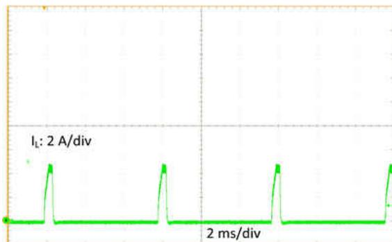
**Figure 8-5. Inductor Current Bursts in Short Circuit**
