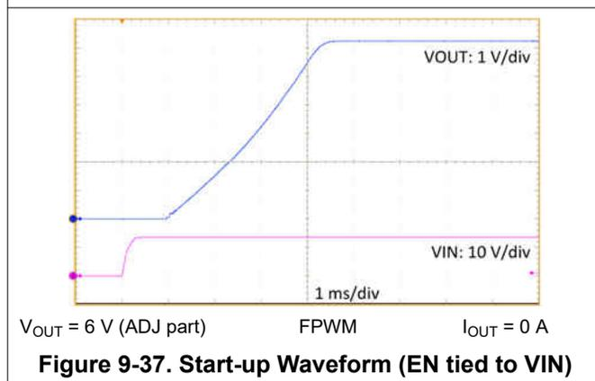
Figure 9-37. Start-up Waveform (EN tied to VIN)
