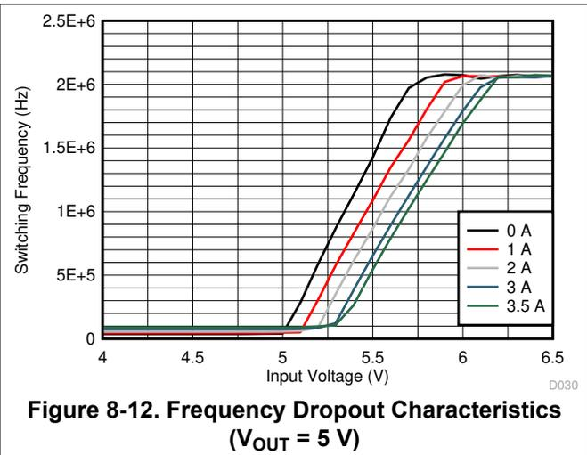
**Figure 8-12. Frequency Dropout Characteristics ( $V_{OUT} = 5\text{ V}$ )**
