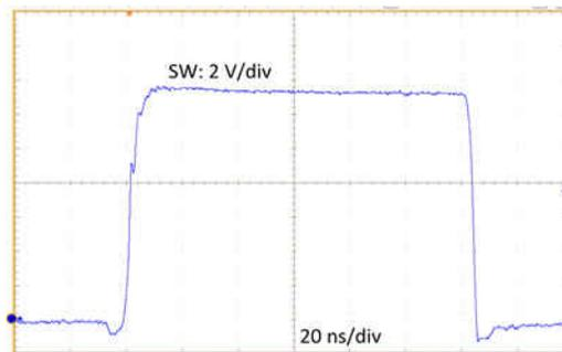
**Figure 8-1. Switch Node Waveform ( $V_{IN}=13.5V$ ,  $I_{OUT}=3.5A$ )**
