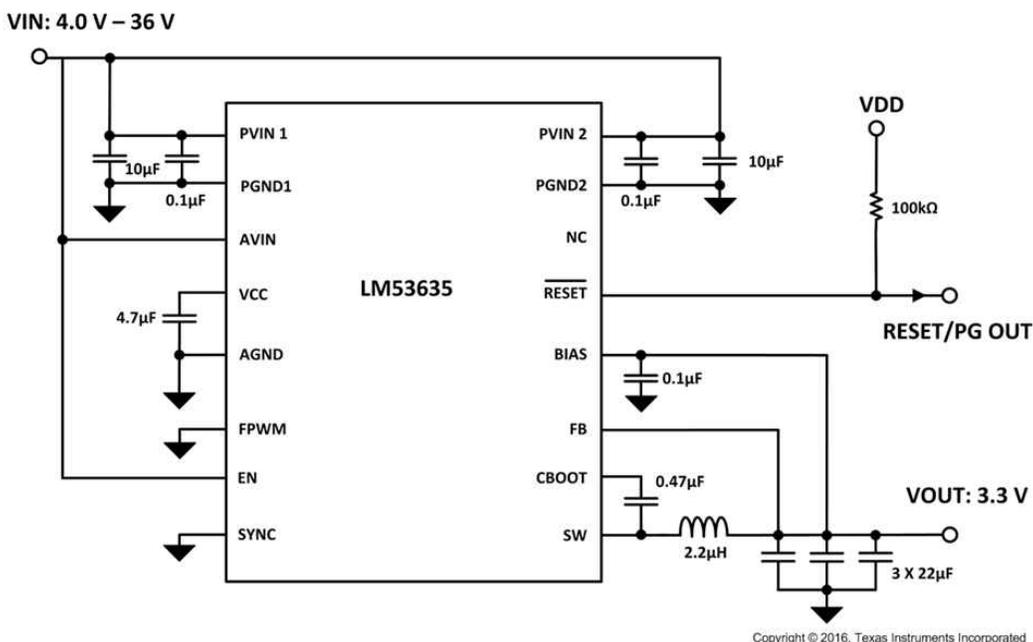
**Figure 9-18. Fixed 3.3-V, 3.5-A Output Power Supply**
