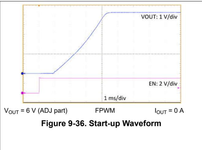
Figure 9-36. Start-up Waveform
