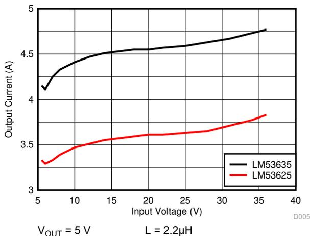
Figure 9-15. Output Current Level Limit Before Overcurrent Protection
