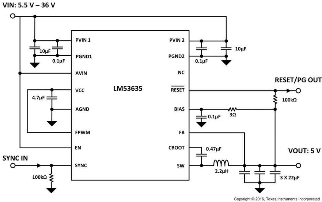
**Figure 9-4. Fixed 5-V, 3.5-A Output Power Supply**
