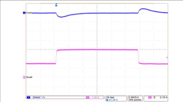
$V_{OUT} = 5\text{ V}$        $F_{SW} = 2100\text{ kHz}$       FPWM mode
