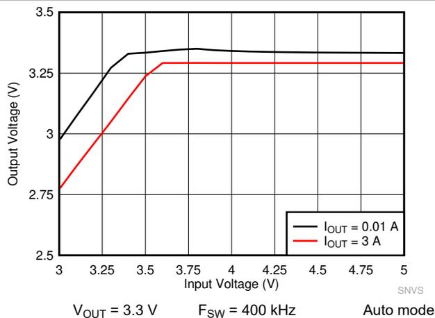
Figure 9-20. LM61430-Q1 Dropout Curve
