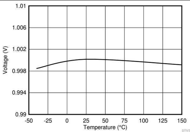
**Figure 7-3. Feedback Voltage**
