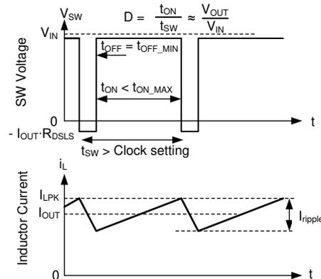
Switching waveforms while in dropout. Inductor current takes longer than a normal clock to reach the desired peak value. As a result, frequency drops. This frequency drop is limited by  $t_{ON\_MAX}$ .
