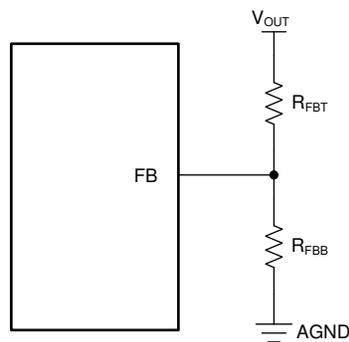
**Figure 8-10. Setting Output Voltage of Adjustable Versions**
