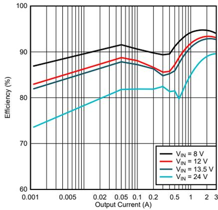
$V_{OUT} = 5\text{ V}$        $F_{SW} = 2100\text{ kHz}$       Auto mode
