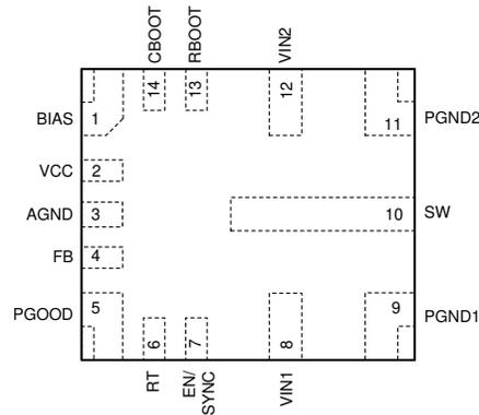
Figure 6-1. RJR Package 14-Pin VQFN-HR (Top View)
