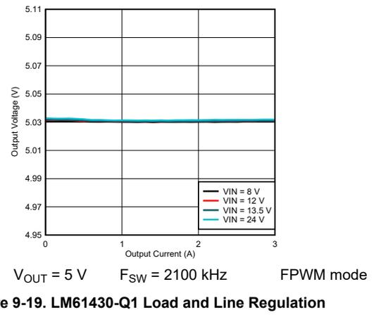
Figure 9-19. LM61430-Q1 Load and Line Regulation
