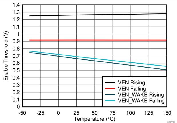
Figure 7-6. Enable Thresholds
