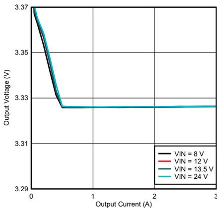
$V_{OUT} = 3.3\text{ V}$        $F_{SW} = 400\text{ kHz}$       Auto mode
