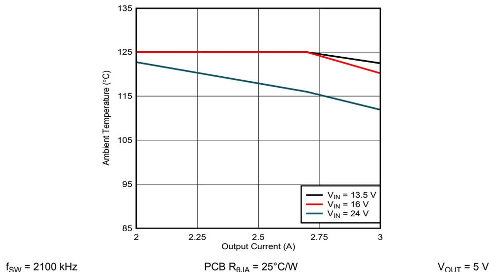
**Figure 9-2. Maximum Ambient Temperature versus Output Current**
