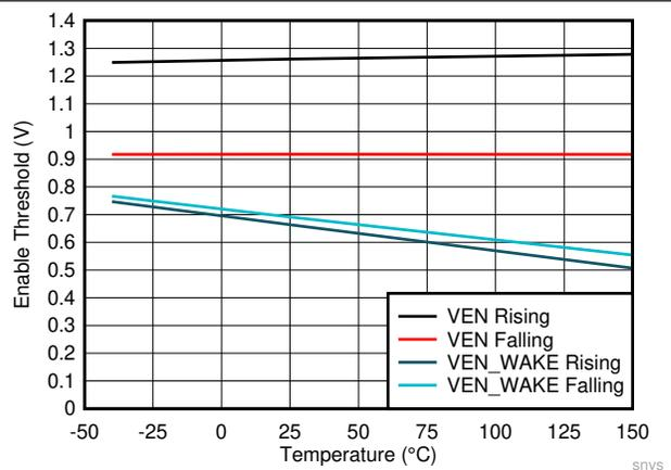
**Figure 7-6. Enable Thresholds**
