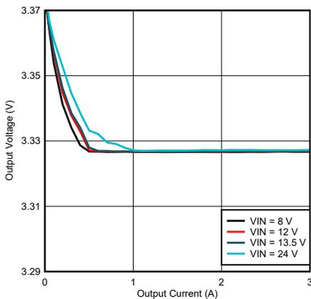
$V_{OUT} = 3.3\text{ V}$        $F_{SW} = 2100\text{ kHz}$       Auto mode
