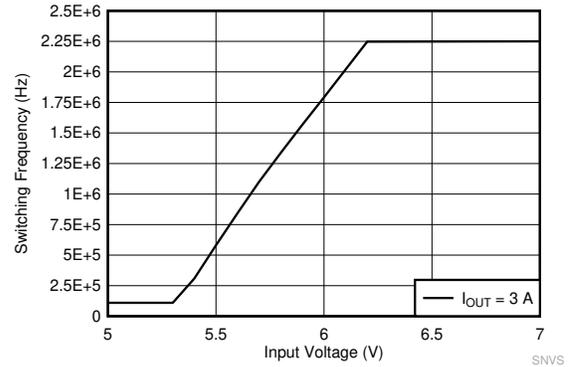
$V_{OUT} = 5\text{ V}$      $F_{SW} = 2100\text{ kHz}$     AUTO Mode
