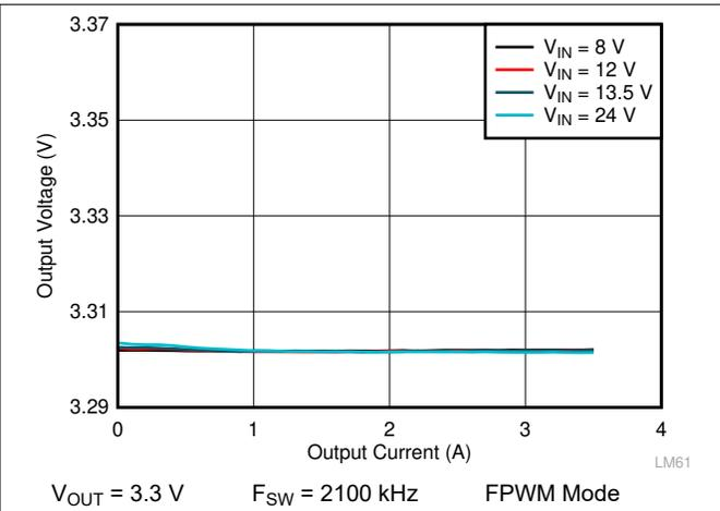
**Figure 9-12. LM61435-Q1 Load and Line Regulation**
