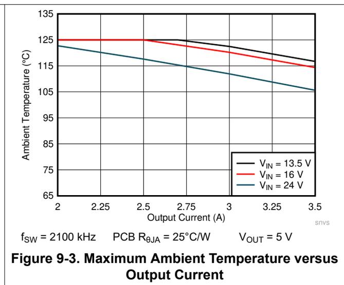
Two other considerations are what maximum and minimum input voltage the part must maintain its frequency setting. Since the LM61435-Q1 adjusts its frequency under conditions in which regulation would normally be prevented by minimum on-time or minimum off time, these constraints are only important for input voltages requiring constant frequency operation.
