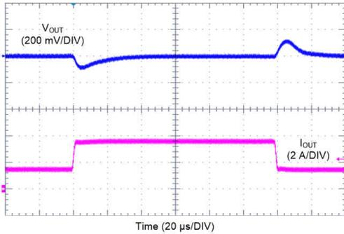
$V_{OUT} = 3.3\text{ V}$        $F_{SW} = 400\text{ kHz}$       AUTO Mode
