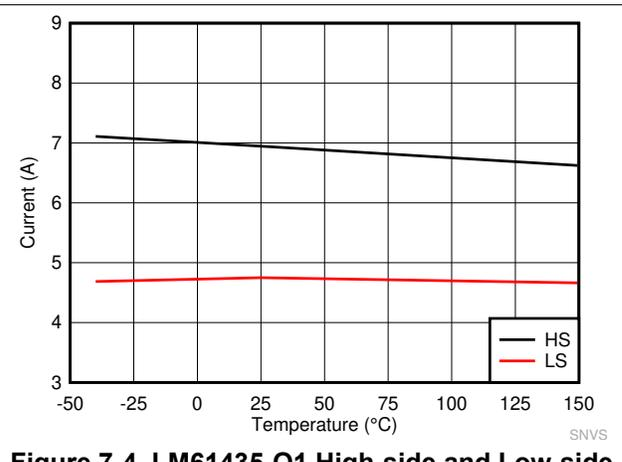
**Figure 7-4. LM61435-Q1 High-side and Low-side Current Limits**
