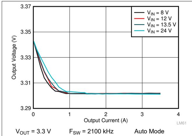
**Figure 9-11. LM61435-Q1 Load and Line Regulation**
