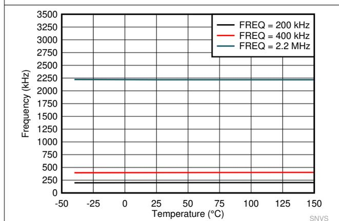
**Figure 7-5. Switching Frequency Set by RT Resistor**
