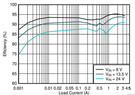
Efficiency  $V_{OUT} = 5\text{ V}$ ,  $F_{SW} = 2200\text{ kHz}$
