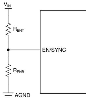
**Figure 8-1.  $V_{IN}$  UVLO Using the EN pin**
