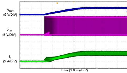
$V_{OUT} = 5\text{ V}$        $F_{SW} = 2100\text{ kHz}$       FPWM Mode
