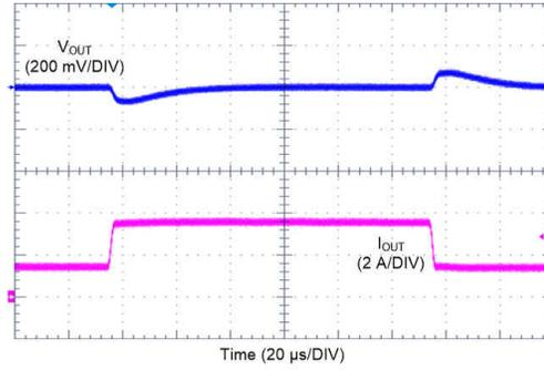
$V_{OUT} = 3.3\text{ V}$        $F_{SW} = 2100\text{ kHz}$       AUTO Mode
