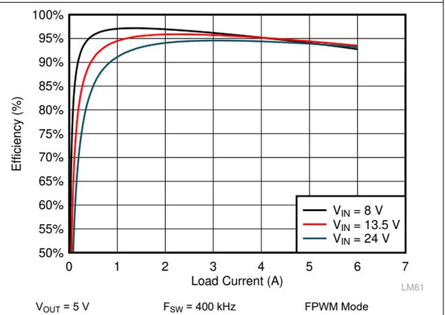
Figure 10-10. LM61460-Q1 Efficiency
