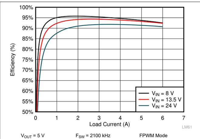
Figure 10-12. LM61460-Q1 Efficiency
