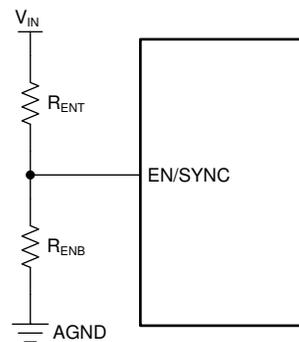
**Figure 9-1.  $V_{IN}$  UVLO Using the EN pin**
