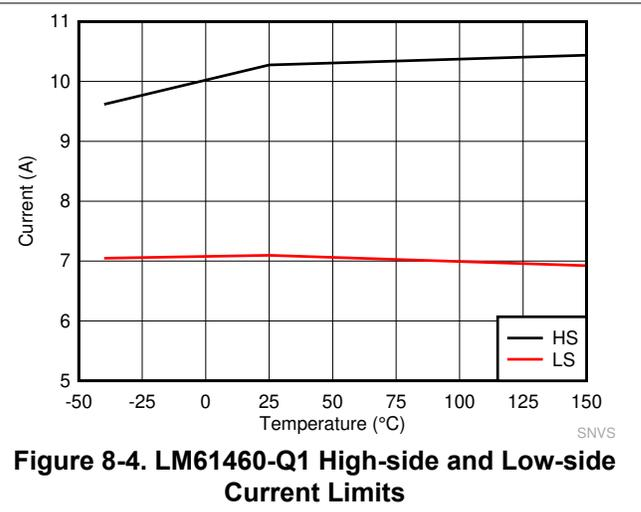
**Figure 8-4. LM61460-Q1 High-side and Low-side Current Limits**
