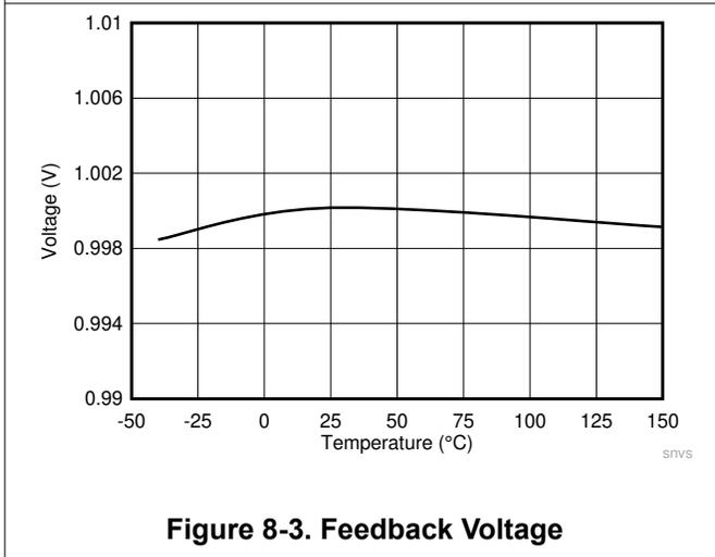
**Figure 8-3. Feedback Voltage**
