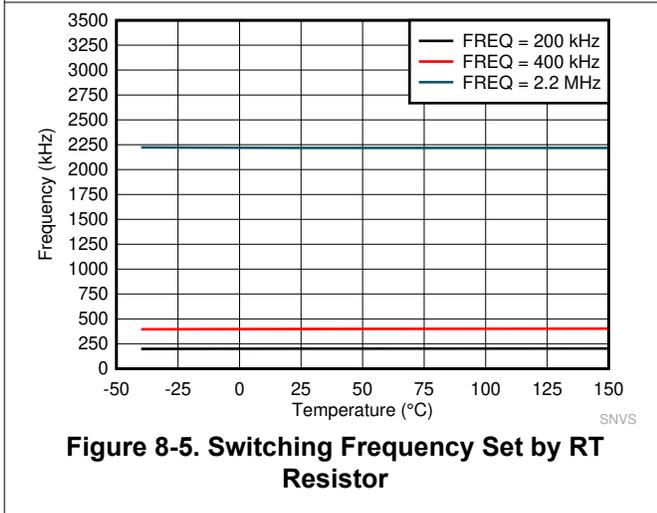
**Figure 8-5. Switching Frequency Set by RT Resistor**
