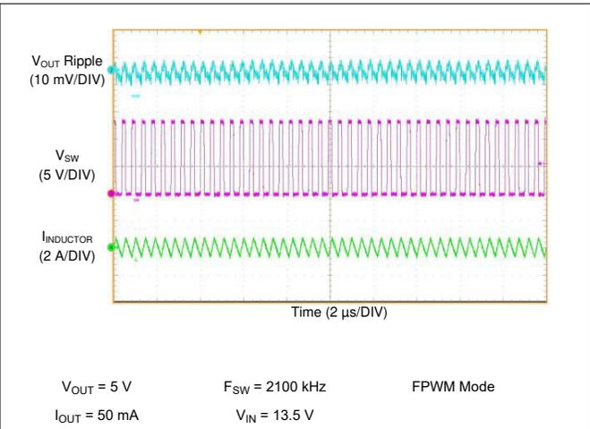
**Figure 10-30. LM61460-Q1 Switching Waveform and  $V_{OUT}$  Ripple**
