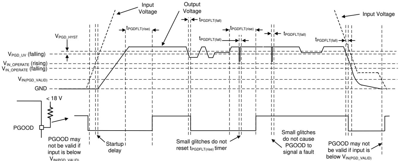
Figure 9-6. PGOOD Timing Diagram (Excludes OV Events)
