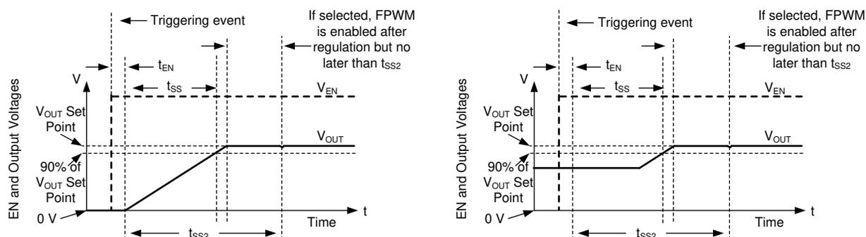
Soft start works with both output voltages starting from 0 V on the left curves, or if there is already voltage on the output, as shown on right. In either case, output voltage must reach within 10% of the desired value  $t_{SS}$  after soft start is initiated. During soft start, FPWM and hiccup are disabled. Both hiccup and FPWM are enabled once output reaches regulation or  $t_{SS2}$ , whichever happens first.
