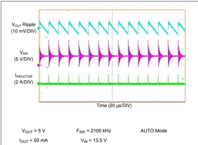
**Figure 10-29. LM61460-Q1 Switching Waveform and  $V_{OUT}$  Ripple**
