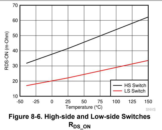
**Figure 8-6. High-side and Low-side Switches  $R_{DS\_ON}$**
