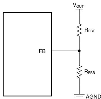
**Figure 9-11. Setting Output Voltage of Adjustable Versions**
