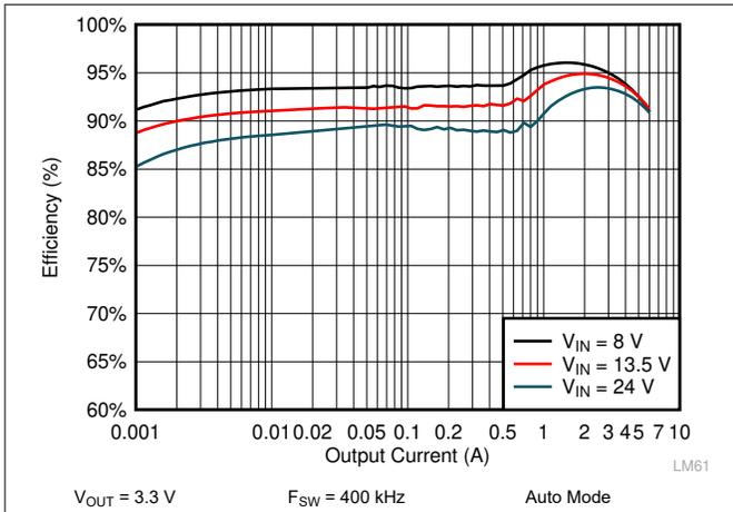
Figure 10-5. LM61460-Q1 Efficiency
