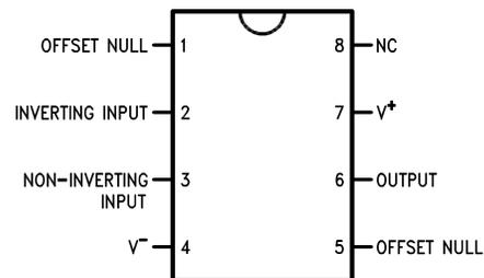
**Figure 2. Dual-In-Line Package**
