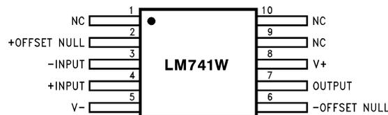
**Figure 3. Ceramic Flatpak and SOIC Package**
