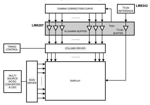
Figure 32. Block Diagram of a Typical TFT-LCD
