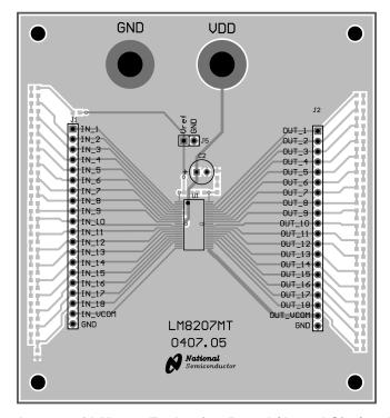
Figure 44. Layout of LM8207 Evaluation Board (Actual Size) — Top View
