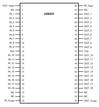
Figure 1. 48-Pin TSSOP Top View
