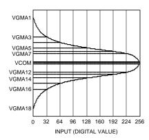
Figure 37. Typical Gamma Correction Curve
