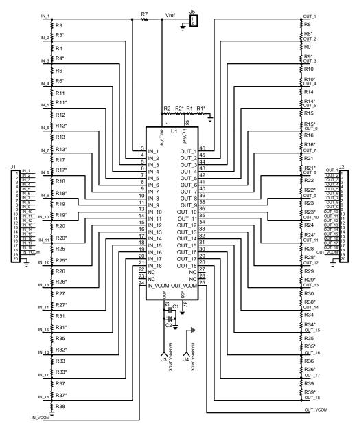
Figure 42. Schematic LM8207 Evaluation Board
