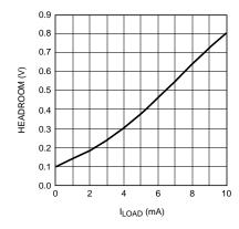
Figure 36. Voltage Reference Headroom vs. Load Current
