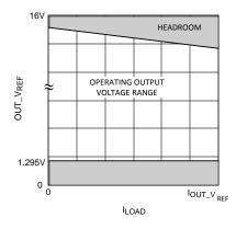
Figure 34. Operating Output Voltage Range
