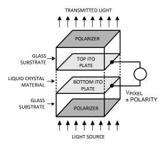
Figure 30. Individual LCD Pixel
