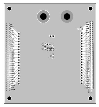
Figure 43. Layout of LM8207 Evaluation Board (Actual Size) — Bottom View
