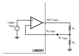
Figure 33. Typical Application Circuit for V<sub>REF</sub>
