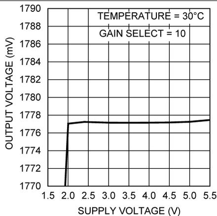
Figure 11. Output Voltage vs. Supply Voltage
