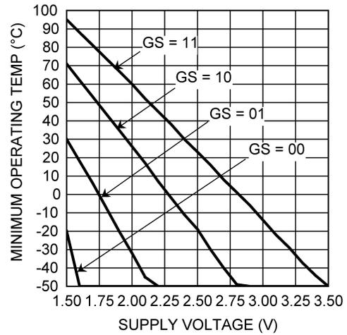
Figure 2. Minimum Operating Temperature vs. Supply Voltage
