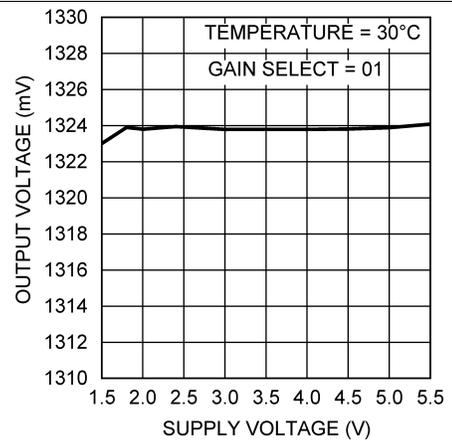
Figure 10. Output Voltage vs. Supply Voltage
