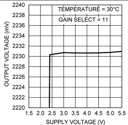
Figure 12. Output Voltage vs. Supply Voltage
