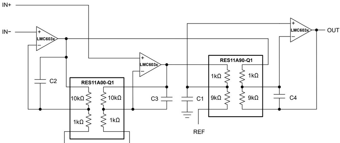
**Figure 6-7. Improved Instrumentation Amplifier With RES11A**
