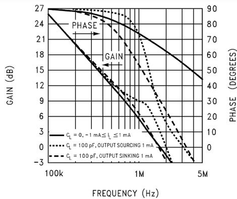
Figure 5-11. Frequency Response vs Capacitive Load
