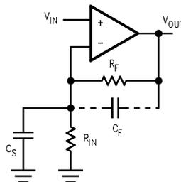
$C_S$  consists of the amplifier input capacitance plus any stray capacitance from the circuit board and socket.  $C_F$  compensates for the pole caused by  $C_S$  and the feedback resistor.
