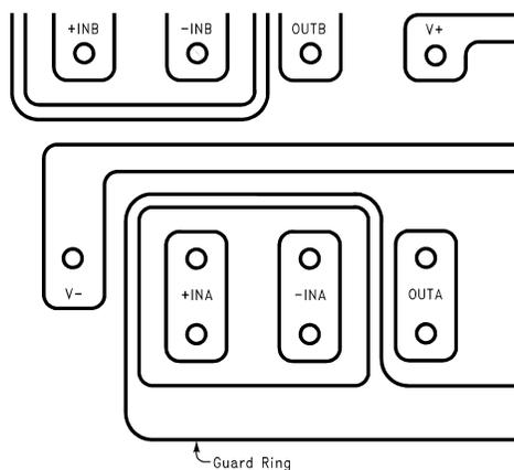
**Figure 6-16. Example of Guard Ring in PCB Layout**
