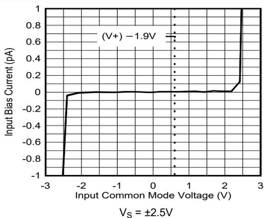
Figure 5-5. Input Bias Current vs Input Common-Mode Voltage
