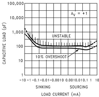
**Figure 5-15. Stability vs Capacitive Load**
