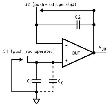
**Figure 6-5. Simple Input Bias Current Test Circuit**
