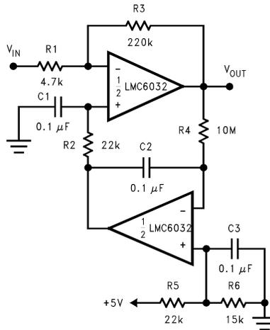
Gain = -46.8 Output offset voltage reduced to the level of the input offset voltage of the bottom amplifier (typically 1mV).
