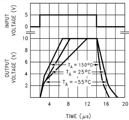
Figure 5-12. Noninverting Large-Signal Pulse Response
