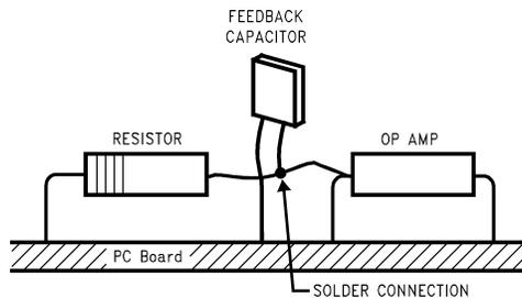
Input pins are lifted out of PCB and soldered directly to components. All other pins connected to the PCB.
