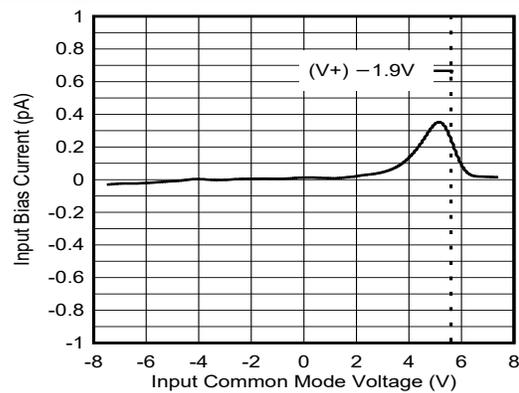
Figure 5-4. Input Bias Current vs Input Common-Mode Voltage
