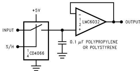
**Figure 6-9. Low-Leakage Sample-and-Hold**
