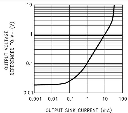
Figure 5-6. Output Characteristics Current Sinking
