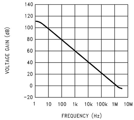
Figure 5-10. Open-Loop Frequency Response
