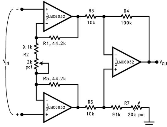
**Figure 6-6. Instrumentation Amplifier**
