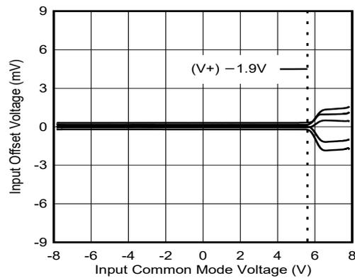
Figure 5-2. Offset Voltage vs Input Common-Mode Voltage
