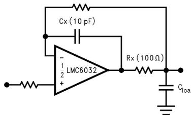
**Figure 6-3. Rx, Cx Improve Capacitive Load Tolerance**
