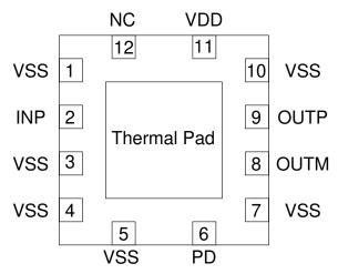
Figure 5-1. RRL Package 12-Pin WQFN Top View
