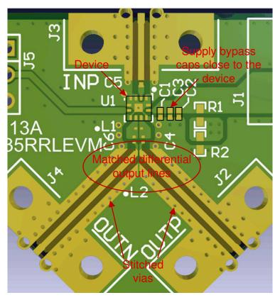
Figure 10-1. Layout Showing Matched Differential Traces and Supply Decoupling
