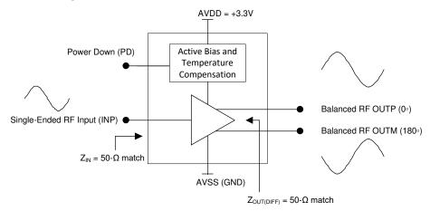
Figure 7-1. Functional Block Diagram
