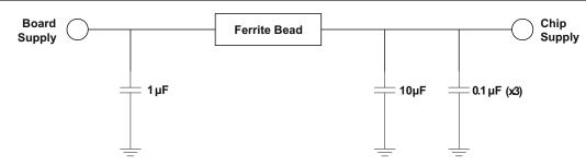
Figure 10-5. Power Supply Decoupling
