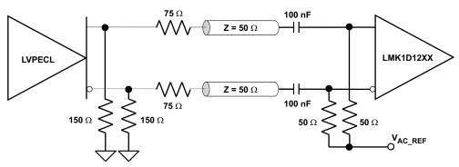
Figure 9-5. LVPECL Clock Driver Connected to LMK1D120x Input
