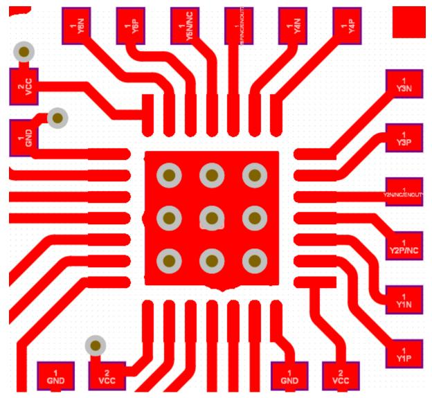
Figure 10-6. Recommended PCB Layout, Top Layer
