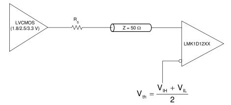
Figure 9-6. 1.8-V/2.5-V/3.3-V LVCMOS Clock Driver Connected to LMK1D120x Input
