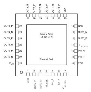
Figure 6-2. LMK1D1208: RHD Package 28-Pin VQFN Top View
