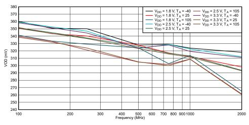
Figure 7-2. LMK1D1208 VOD vs. Frequency
