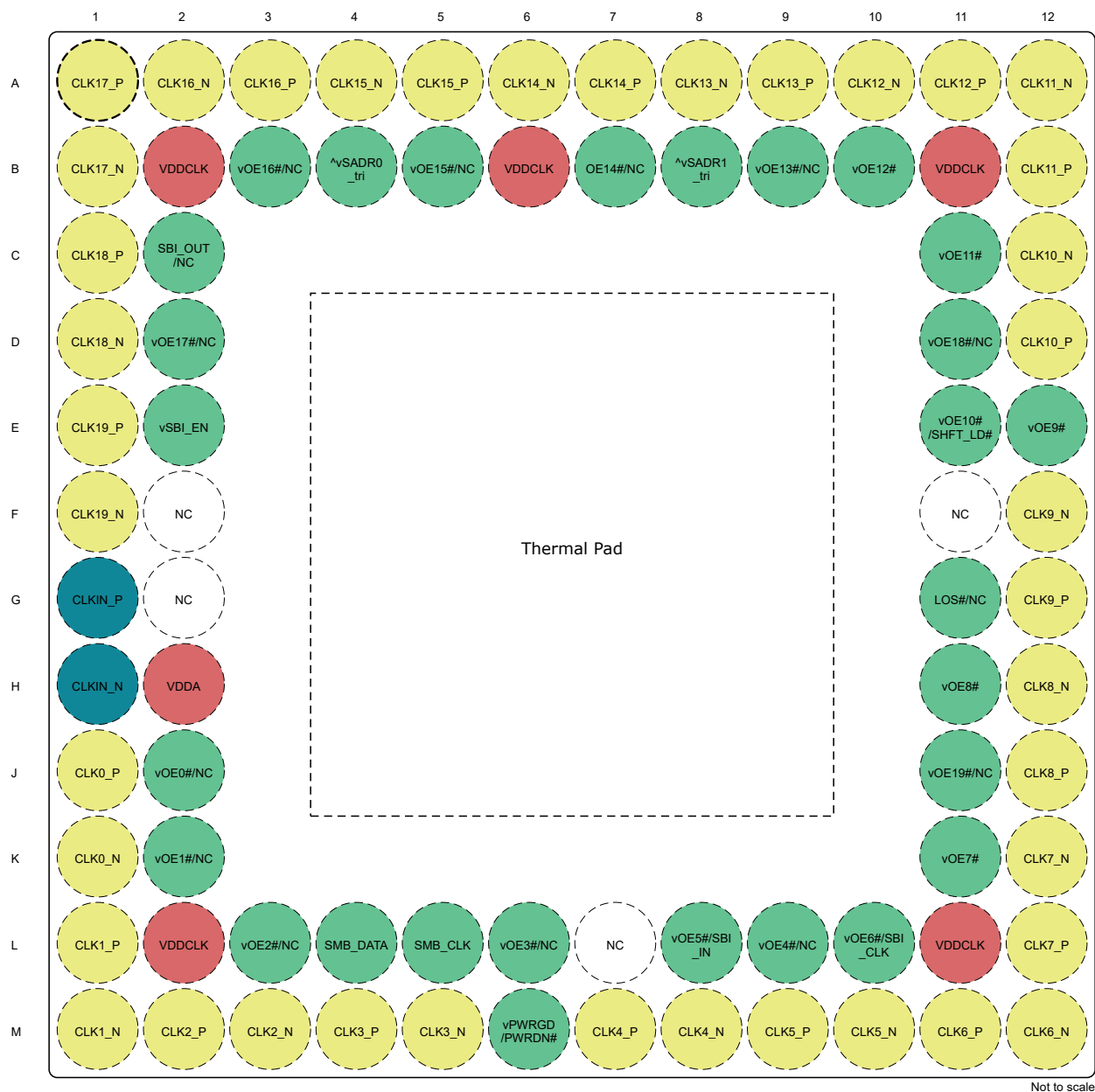
Figure 5-1. LMKDB1120 and LMKDB1120FS 6mm × 6mm NPP Package 80 Pin TLGA Top View
