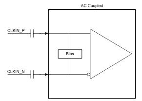
Figure 8-4. External AC-Coupled Input
