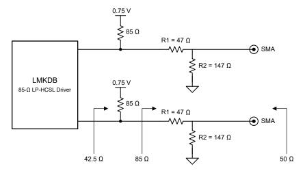
Figure 7-3. DB2000QL DC Test Load
