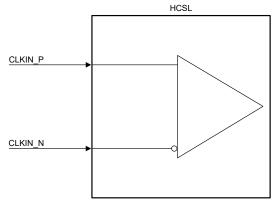
Figure 8-2. HCSL Input Interface (PCIe Standard)
