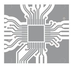
Figure 10-3. LMKDB1204 Layout Example - Bottom Layer
