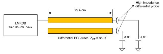
Figure 7-2. DB2000QL AC Test Load
