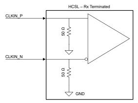
Figure 8-5. Receiver Internal Terminations
