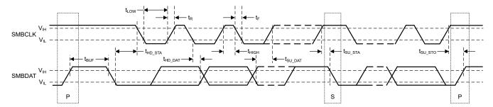
Figure 6-1. SMBus Timing Diagram
