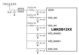
Figure 10-2. Power Supply Recommendation for LMKDB12XX MUX
