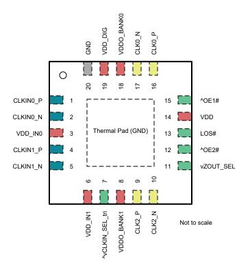
Figure 5-2. LMKDB1202 3mm × 3mm VQFN Package 20 Pin Top View
