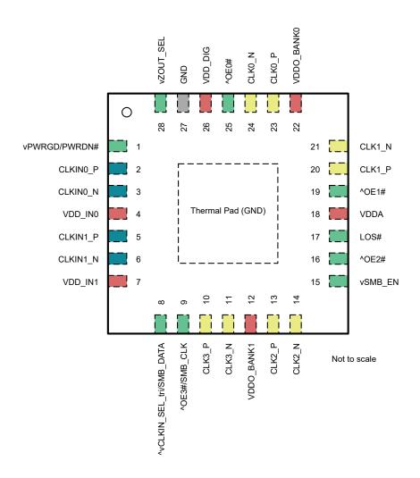
Figure 5-1. LMKDB1204 4mm × 4mm VQFN Package 28 Pin Top View
