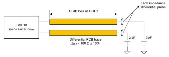
Figure 7-1. PCle AC Test Load
