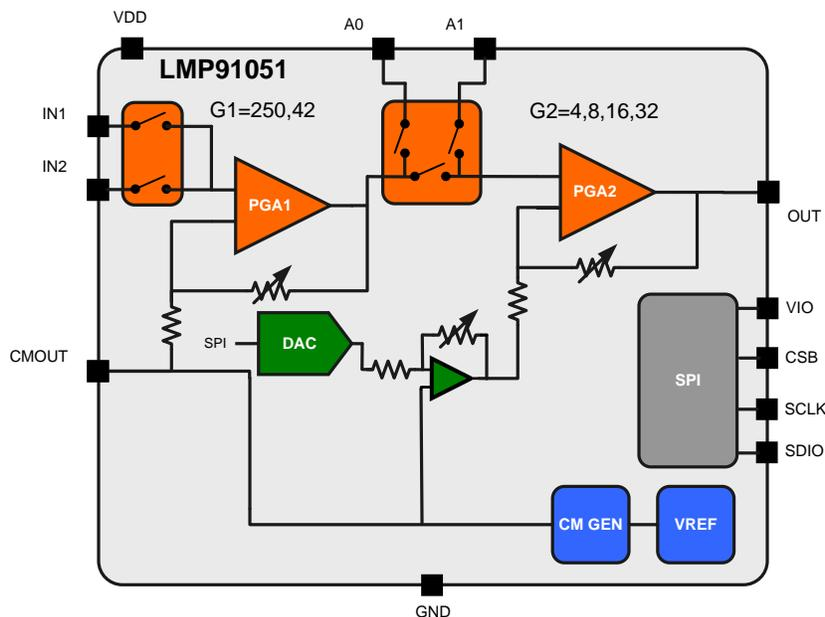
Figure 14. LMP91051 Sensor AFE for NDIR Sensing
