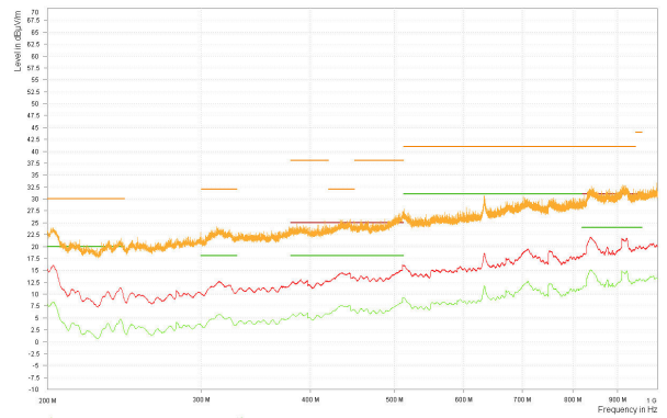
V_{OUT} = 3.3V F_{SW} = 2MHz I_{OUT} = 1A Frequency span: 200MHz to 1GHz
