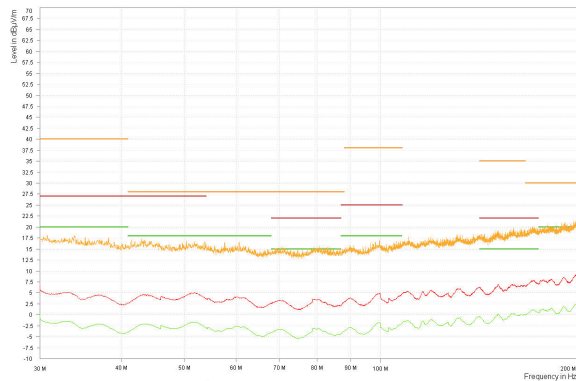
V_{OUT} = 3.3V F_{SW} = 2MHz I_{OUT} = 1A Frequency span: 30MHz to 200MHz
