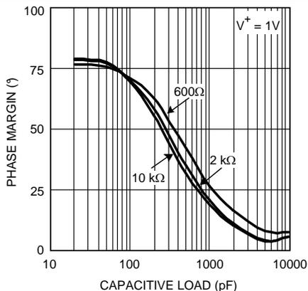
Figure 37. Phase Margin vs Capacitive Load (Stability)
