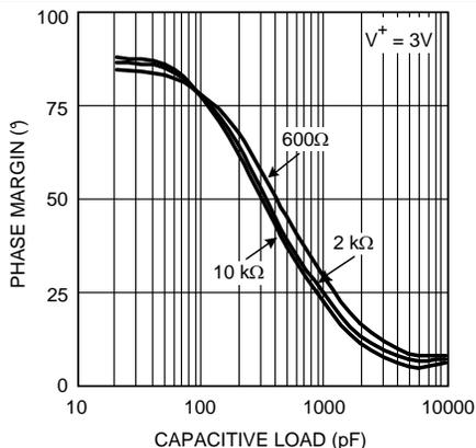
Figure 39. Phase Margin vs Capacitive Load (Stability)
