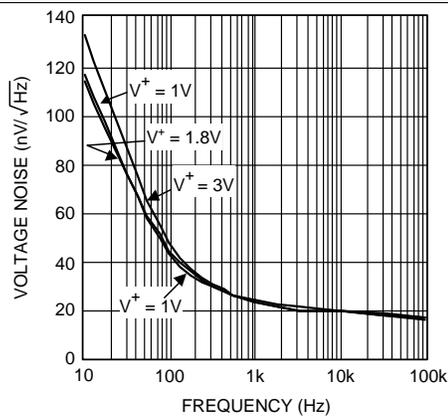
Figure 42. Input Referenced Voltage Noise vs Frequency
