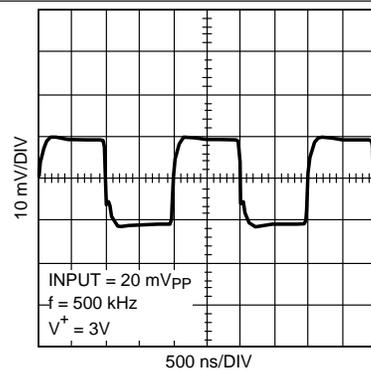
**Figure 35. Small Signal Transient Response,  $A_V = +1$**
