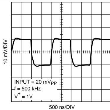
**Figure 31. Small Signal Transient Response,  $A_V = +1$**
