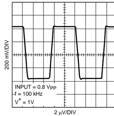
**Figure 32. Large Signal Transient Response,  $A_V = +1$**
