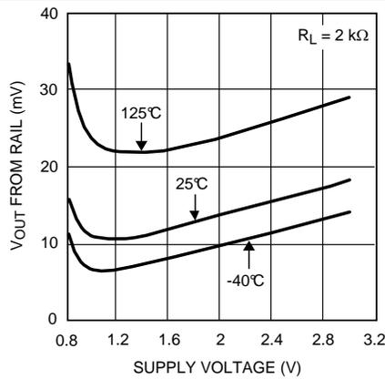
Figure 21. Positive Output Swing vs Supply Voltage
