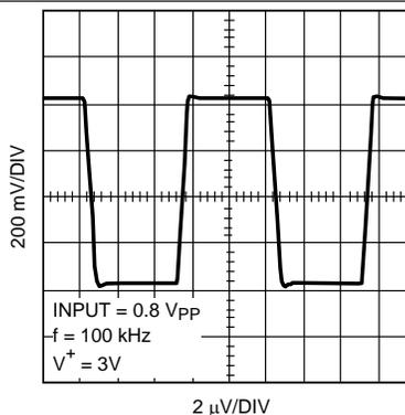
**Figure 36. Large Signal Transient Response,  $A_V = +1$**
