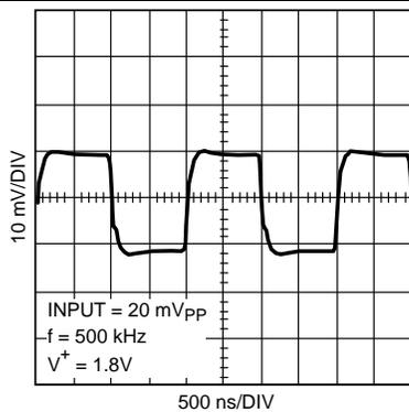
**Figure 33. Small Signal Transient Response,  $A_V = +1$**
