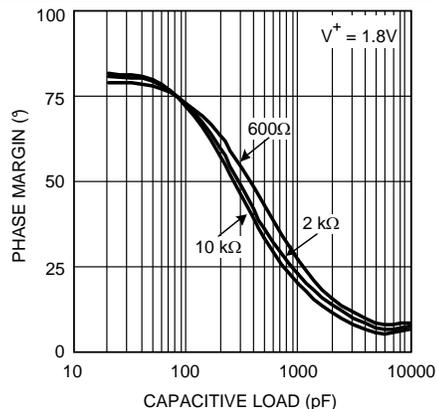
Figure 38. Phase Margin vs Capacitive Load (Stability)
