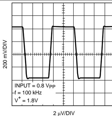
**Figure 34. Large Signal Transient Response,  $A_V = +1$**
