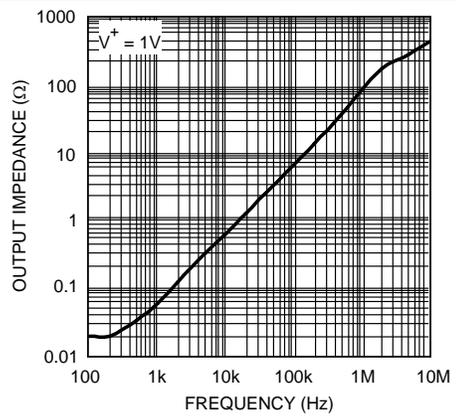
**Figure 46. Closed Loop Output Impedance vs Frequency**
